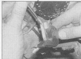
12.3b ... then draw the cable from the housing ...
