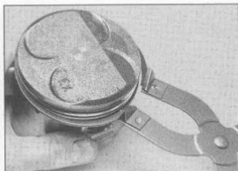
15.5 Removing the piston rings using a ring removal and installation tool
