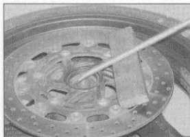
16.3 Lever out the grease seal on each side
