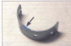
5.14 Shell bearings are either plain or grooved. They are usually identified by colour code (arrow)
