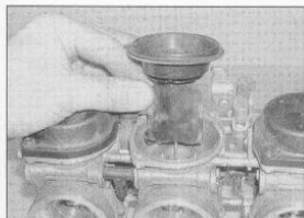
10.29d Install the piston/diaphragm assembly ...
