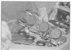
7.9 Lift the carburetors off the intakes and remove them
