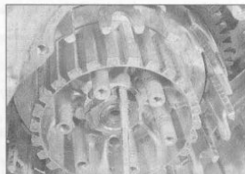
17.7a Bend back the lockwasher tabs ...
