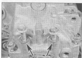
23.20 The two 9 mm bolts on each end (arrowed) have steel washers
