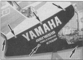
3.10 Lower fairing fasteners (arrowed)
