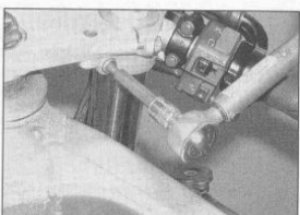
20.15c ... then tighten the clamp bolts to the specified torque
