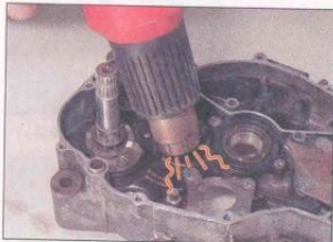
2.15 Using heat to free a seized fastener
