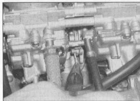
11.3f ... and detach the cable end from the carburettor
