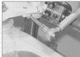
6.9c . . . and the handlebar clamp bolt(s) to the specified torque
