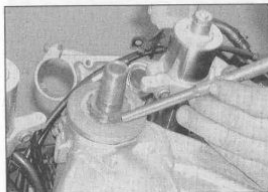
20.12 If the tool is not available, adjust the bearings as described
