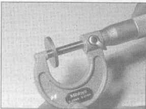
Tappet shims are measured with a micrometer
