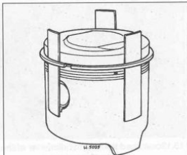
16.12 Old pieces of feeler gauge blade can be used to guide the ring over the piston
