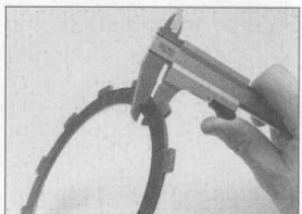
17.12 Measuring clutch friction plate thickness
