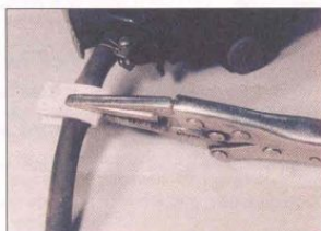
9.4 ... or thick card and self-locking grips
