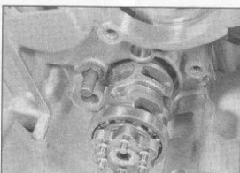
31.6 Withdraw the selector drum from the crankcase
