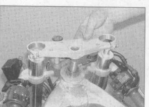
18.7c ... and ease the yoke up off the steering stem and forks
