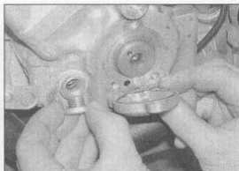
27.17 Install the end-cover and plug using new O-rings
