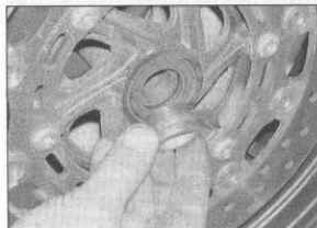
14.6a Remove the spacer . . .
