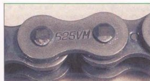
8.10 Typical chain size and type marking
