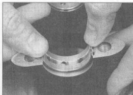
28.28 Make sure the tabs on the shells locate in the notches in the cutouts
