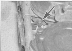
10.1a Make sure the slot in each arm locates correctly behind the nipple on the end of each choke plunger (arrowed)
