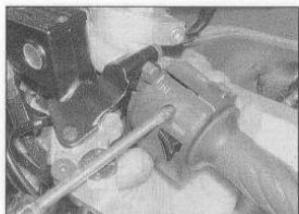
12.4a Remove the housing screws and separate the halves
