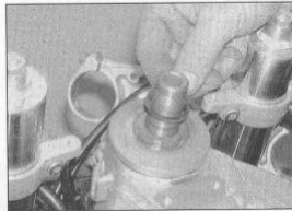
20.10c . . . and remove the rubber washer
