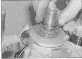
20.10a Remove the tabbed lockwasher . . .
