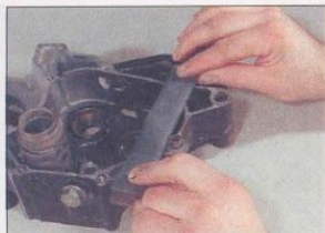
7.6 Fine abrasive paper is wrapped around a flat file to clean up the gasket face
