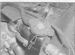
16.6c Pressure cap (arrowed) – YZF750R and SP models
