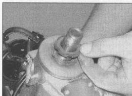
8.8a Unscrew the adjuster nut ...
