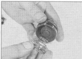
18.41 Fit the narrow end of the spring over the lug on the piston
