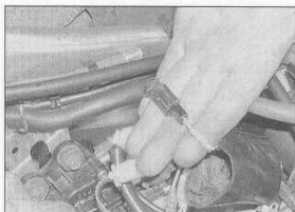
14.3c Rear brake switch wiring connector – YZF1000R models
