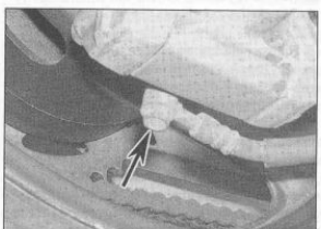
7.2b Brake hose banjo bolt (arrowed)
