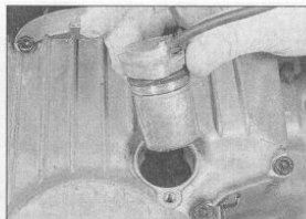
26.10 Use a new O-ring when installing the sensor
