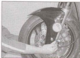
20.4 Checking for play in the steering head bearings
