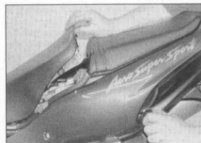
2.3a Turn the key and draw the seat up and back ...
