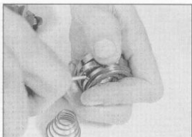
18.37 Remove the seal from the piston using a non-metallic tool
