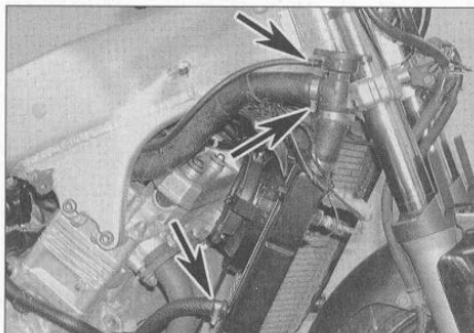
7.4a Release the clamps and detach the hoses (arrowed) from the right-hand side ...
