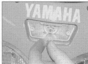
7.7c Pull the bulb out of the bulbholder
