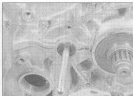
17.5c The pushrod can be withdrawn from the left
