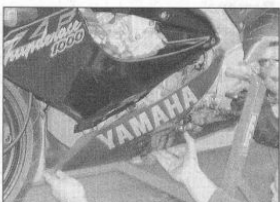
3.29d ... and remove the lower fairing, noting how it fits
