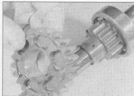
30.48a Slide the 4th gear pinion ...
