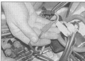
22.2b Sidestand switch wiring connector – YZF1000R models
