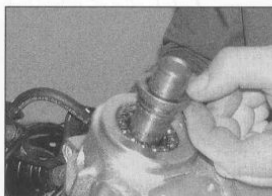
8.12b ... and its inner race into the steering head
