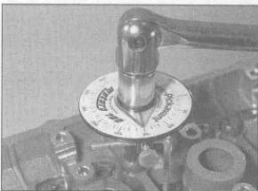
Angle-tightening cylinder head bolts
