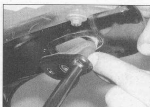
4.2b ... and the rubber pad if required
