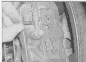
2.2a Insert the pad pins ...
