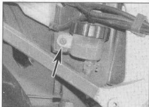
9.4a Remove the screw (arrowed) and drain the reservoir ...
