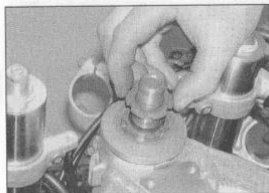
20.10b . . . then unscrew the locknut . . .
