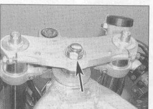
18.7b ... then unscrew the steering stem nut (arrowed) ...
