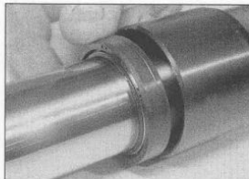
7.24 Drive the oil seal into the bottom of the outer tube ...
