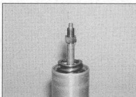
7.28b Tie a piece of wire around the damper cartridge as shown and use it to keep the cartridge extended
