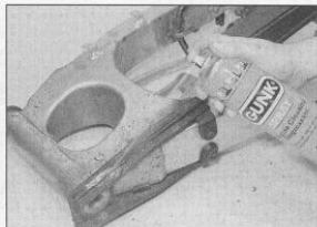
14.1 Clean off all accumulated chain lube and road dirt using a suitable degreaser
