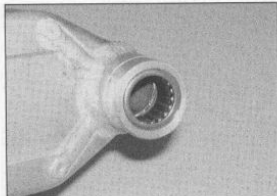
14.3 Check the needle bearing in each side as described
