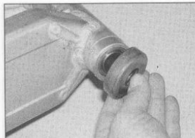
14.2a Remove the cap and washer(s) . . .
