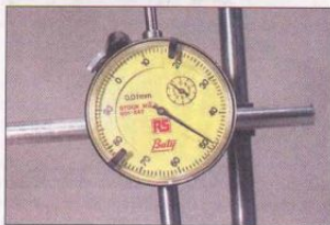
3.17 Dial gauge reading of 1.48 mm
