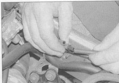
4.6c ... and connect the gauge hoses using suitable unions
