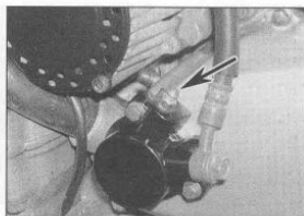
19.5 Clutch release system bleed valve (arrowed)
