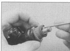
9.9 Remove the dust boot from the bottom of the master cylinder
