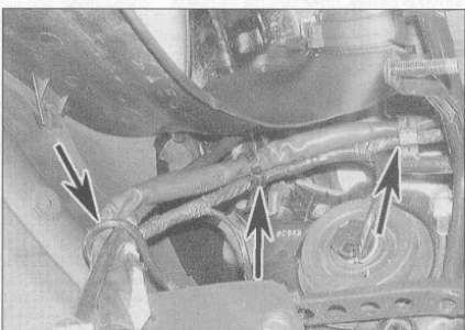
15.3a Release the wiring from its clips and ties (arrowed) ...
