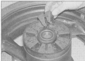
16.15b . . . and remove the rubber damper segments
