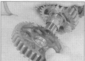
30.62b ... and the 1st gear pinion onto the shaft ...
