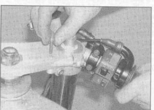
18.6b ... and unscrew the positioning bolts
