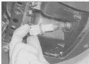
7.8a Release the bulbholder from the base of the headlight
