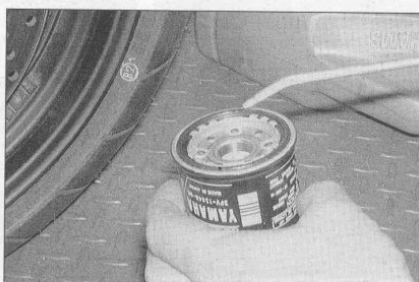
21.3a Smear some clean oil onto the seal ...
