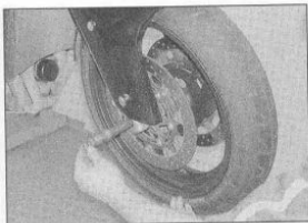
14.11b ... and insert the axle
