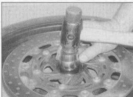
16.10 A socket can be used to drive in the bearing
