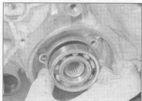
32.5a Remove the bearing . . .
