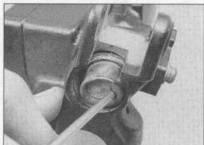
5.10c Remove the rubber boot from the end of the master cylinder piston ...
