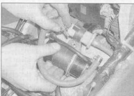
5.7c ... then unscrew the bolt and remove the pump/filter assembly
