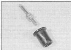
18.10 Draw the pushrod and the rubber boot out of the cylinder
