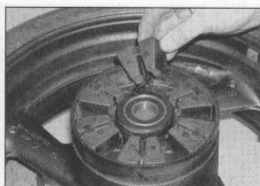
17.3 ... and remove the rubber dampers
