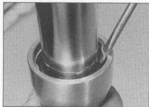
7.45 ... then lever out the retaining clip using a flat-bladed screwdriver
