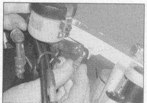
8.3 Displace the reservoir(s) from the top yoke ...
