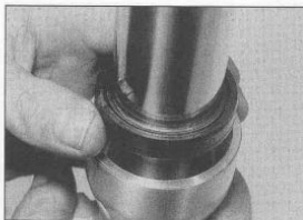
7.56 Make sure the oil seal is the correct way up
