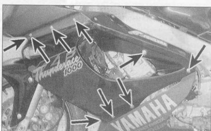
3.26b Fairing side panel fasteners (arrowed)
