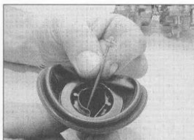
10.29b ... then fit the needle into the piston ...
