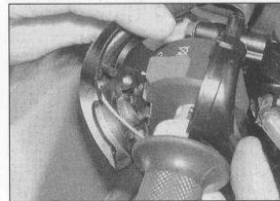
11.4c Separate the housing halves ...
