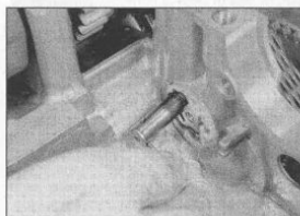
24.2c ... then withdraw the nozzle
