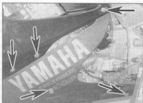
3.29c Remove the screws (arrowed) ...
