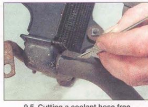
9.5 Cutting a coolant hose free with a sharp knife
