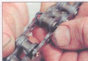
8.3 ... and separate the chain link
