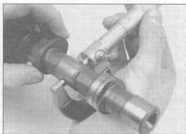
10.16b Measure the cam bearing journals with a micrometer
