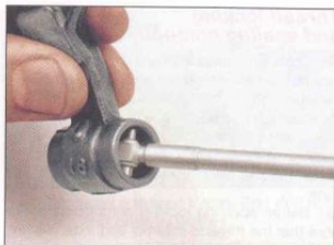
3.7 Expand the telescoping gauge in the bore, lock its position ...
