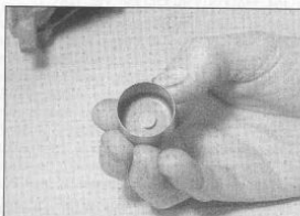
27.12b ... and remove the shim from inside the follower
