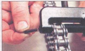
8.2 ... withdraw the pin, remove the tool ...
