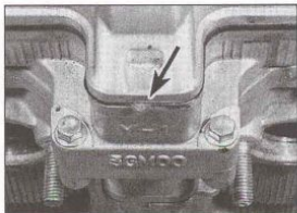
8.7 The tab on the gasket must be at the front of the cover
