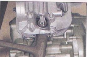
7.2 Tap around the joint with a soft-faced mallet if necessary - don't strike cooling fins
