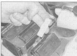
5.6 Disconnect the negative wire wiring connector
