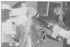
18.4 Disconnect the clutch switch wiring connector (arrowed) – YZF1000R model shown
