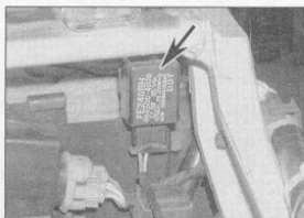
11.3b Turn signal relay – YZF1000R models
