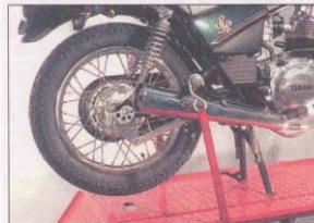
1.2 Tie-downs are used around the passenger footrests to secure the bike
