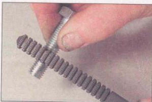
2.24 Using a thread restorer file
