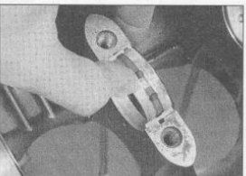
28.3 To remove a main bearing shell, push it sideways and lift it out
