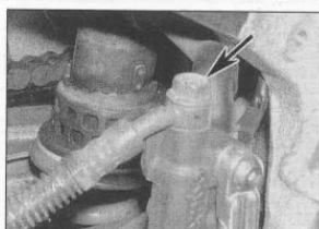
9.5 Brake hose banjo bolt (arrowed)
