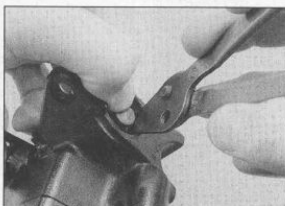
5.11 ... then depress the piston and remove the circlip using a pair of internal circlip pliers
