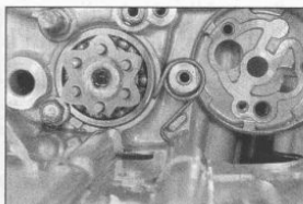
20.10a Fit the return spring as shown ...
