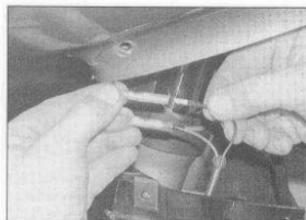
3.27a Disconnect the turn signal wiring connectors
