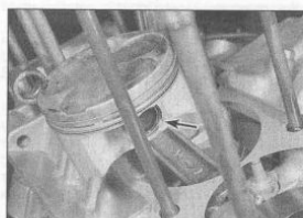
15.17 Do not over-compress the circlips and make sure they seat in the groove (arrowed)
