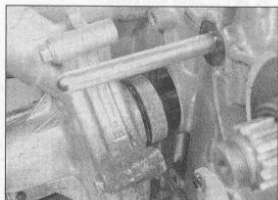
8.7b ... and withdraw the pump from the crankcase, bringing the pipe with it
