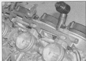
10.22b ... and install the linkage bar, making sure the slots in the arms locate behind the nipples on the plungers
