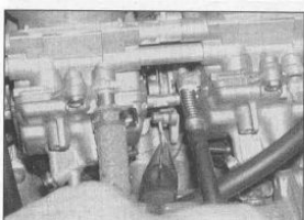
11.3f ... and detach the cable end from the carburettor
