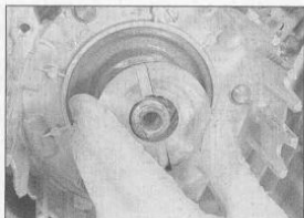
17.8b ... and remove the outer thrust plate
