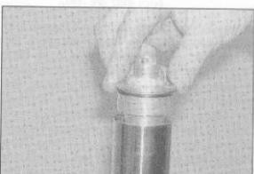
7.62 Thread the top bolt into the fork tube
