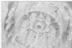
17.8a Slide the clutch centre (arrowed) off the shaft ...
