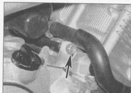
3.3c Idle speed adjuster screw (arrowed) - YZF1000R and 750 SP models
