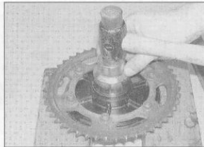
16.29 A socket can be used to drive in the bearing
