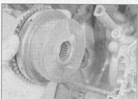
32.6 Disengage the chain and remove the starter clutch
