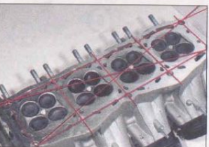
3.23 Check for warpage in these directions
