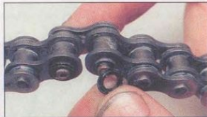
8.5 ... install the O-rings over the pin ends ...
