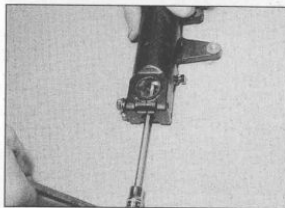
7.2 Slacken the damper rod Allen bolt
