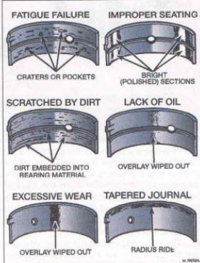
5.17 Typical bearing failures
