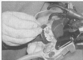
11.4e ... and free the cable ends from the throttle pulley
