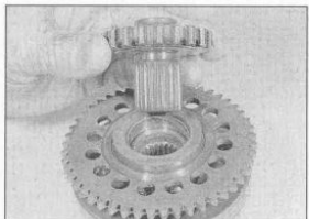
32.8a Withdraw the sprocket
