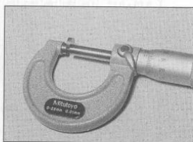
27.13 Measure the shim using a micrometer
