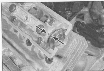
27.5c Align the punchmark on each camshaft with the mark on the holder (arrowed)
