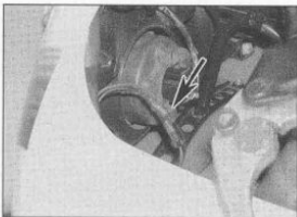
3.6a Disconnect the turn signal wiring connectors (arrowed)
