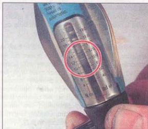
4.1 Set the torque wrench index mark to the setting required, in this case 12 Nm
