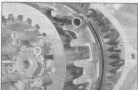
17.26a Fit a friction plate first then a plain plate and so on
