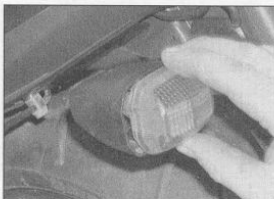
12.3 Make sure the tab locates correctly when fitting the lens
