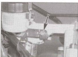
20.6a Unscrew the brake reservoir bolt (arrowed) ...
