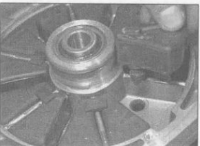
Cush drive rubbers dampen out transmission shocks
