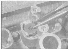
10.21a Fit the shim into the recess in the top of the valve ...
