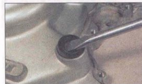
6.1 Prise out oil seals with a large flat-bladed screwdriver
