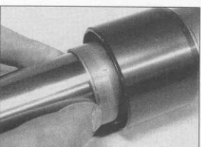
7.22 Make sure the bottom bush enters the outer tube squarely
