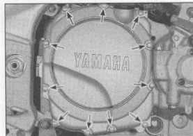
17.3 Unscrew the bolts (arrowed) and remove the cover
