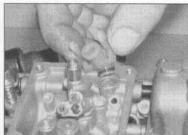
10.4a Press the needle valve seat into place
