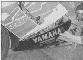
3.11 Note how it engages with the side panel
