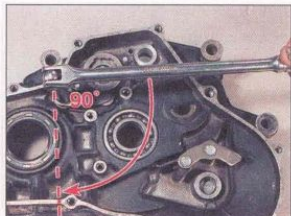
4.3 ... or by marking the angle on the surrounding component
