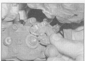
14.3b Draw the pulley off the shaft and detach the cable nipples ...
