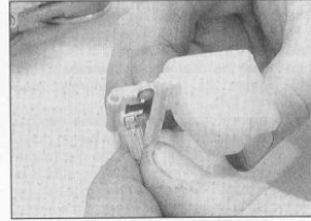
10.24c Hook the needle valve onto the tab on the float ...
