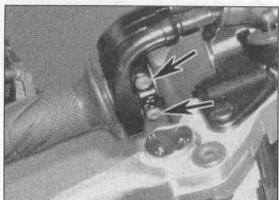
11.4b ... and remove the housing screws (arrowed)
