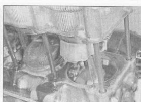
14.3 Lift the block up off the studs
