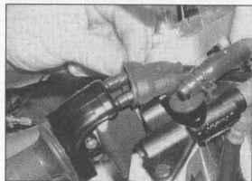
11.4a Pull the boot back off the housing ...
