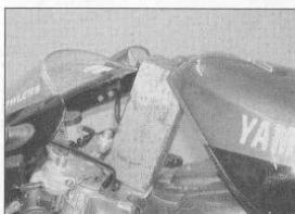
2.9 Raise the front of the tank and support it
