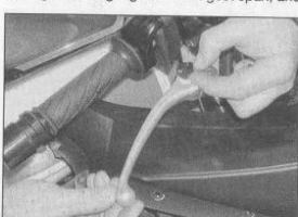
9.6 Adjusting the front brake lever span
