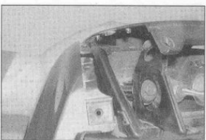
10.2c ... then remove the taillight/bracket/top cover assembly, noting how it fits
