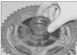
16.31a Press or drive the seal into the coupling . . .
