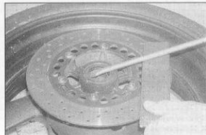
16.17 Lever out the grease seal
