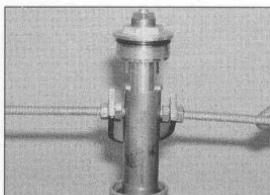
7.5b Fit the tool into the holes in the spacer as shown
