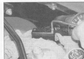
18.3b Slacken the reservoir cover screws
