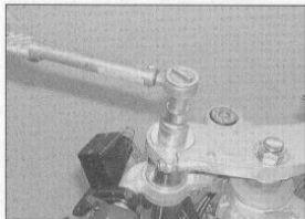
6.9a If slackened, tighten the fork top bolt to the specified torque
