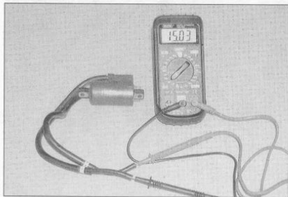
3.7 To test the coil secondary resistance, connect the multimeter leads between the spark plug leads
