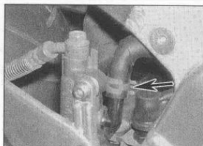
9.4b ... and detach the hose (arrowed) from the master cylinder
