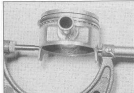
15.12 Measure the piston diameter with a micrometer at the specified distance from the bottom of the skirt
