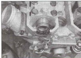
8.8 Apply the sealant to the cutouts in the head
