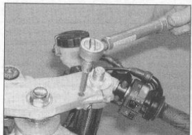
20.15b ... and tighten it to the specified torque ...
