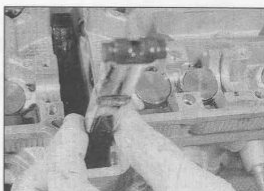
9.16 Lift the front guide out of the engine noting how the lugs locate in the cutouts
