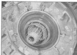
17.23b ... and the needle bearing into the middle of the housing
