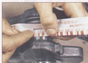
3.16 Measuring the width of the crushed Plastigauge
