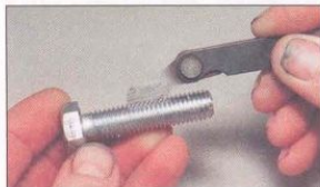
2.12 Using a thread gauge to measure pitch
