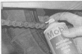
1.15 Apply the lubricant to the overlap between the sideplates
