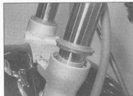
19.3b . . . and check underneath it for signs of oil leakage
