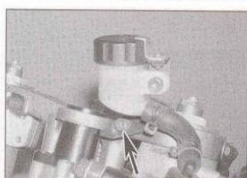
20.6b ... and on 750's the clutch reservoir bolt (arrowed) and displace them
