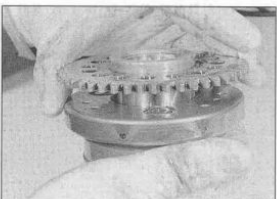
32.8b Check the operation of the clutch as described
