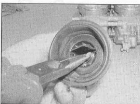
8.24c Pull the jet needle holder out of the piston
