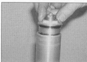
7.32 Thread the top bolt into the fork
