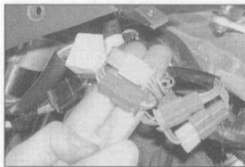
19.3a Left-hand switch wiring connectors (arrowed) – YZF1000R model shown
