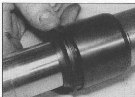
7.25b ... then press the dust seal into place
