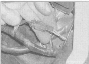
14.3b Rear brake switch wiring connector – YZF750R and SP models
