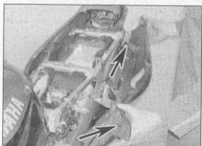
3.24b ... and release the pegs (arrowed) from the grommets ...
