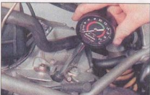
3.20 Using a rubber-cone type cylinder compression gauge
