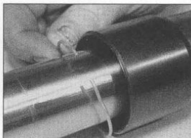
7.25a ... and fit its retaining clip, making sure it is properly seated ...
