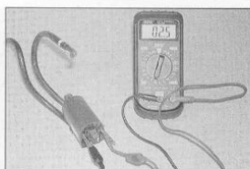
3.6 To test the coil primary resistance, connect the multimeter leads between the primary circuit terminals
