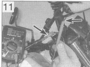
Continuity check of front brake light switch sub-harness
