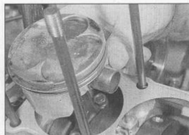
15.3b . . . then push out the pin and remove the piston
