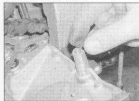
16.11b ... and the small gasket, using a dab of grease to hold it ...
