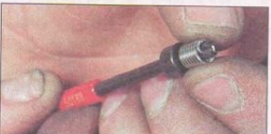
2.28 ... fit insert on the installing tool ...
