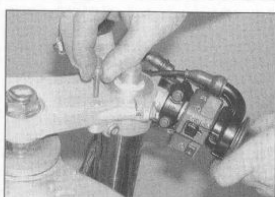
20.15a Align the handlebar, then install the bolt ...
