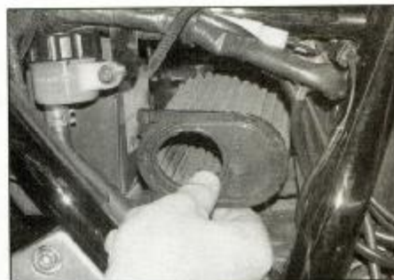
5.2c . . . and withdraw the element
