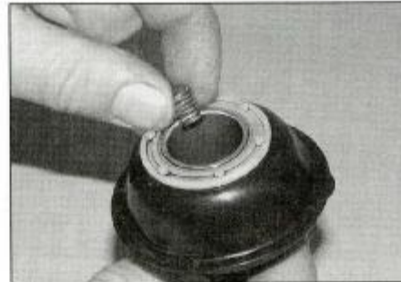
10.8e . . . then fit the spring onto the needle
