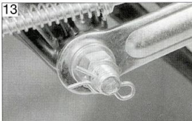
13 Brake torque arm must be properly secured at both ends
