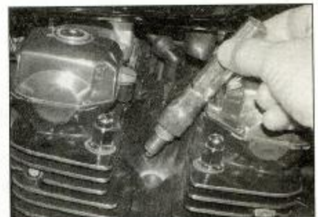
2.9 Thread the plug as far as possible turning the tool by hand
