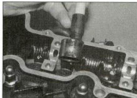
11.10 Lift out the follower using a magnet or valve lapping tool if necessary
