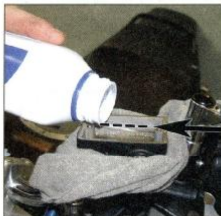
3 Top up with fluid of the recommended type until the level is up to the ridge along the inside of the front wall of the reservoir (arrowed). Do not overfill.
