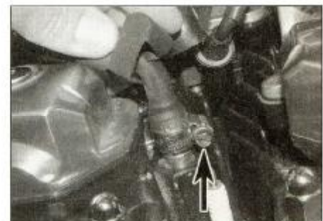
16.5b Slacken the clamp screw (arrowed) on each pipe and detach them from their unions
