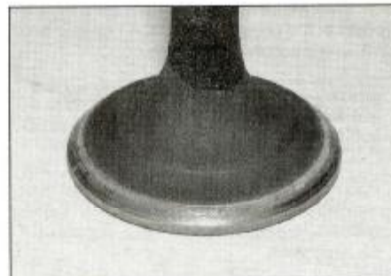
14.24b The valve face and seat should show a uniform unbroken ring
