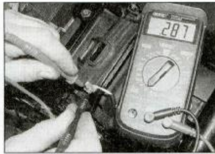
4.4 Measuring pick-up coil resistance
