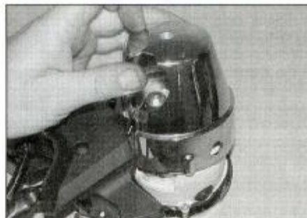
16.4b . . . and remove the chrome covers
