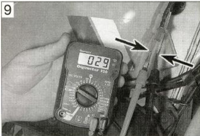
9 Continuity check of front brake light switch using a meter - note split pins used to access connector terminals
