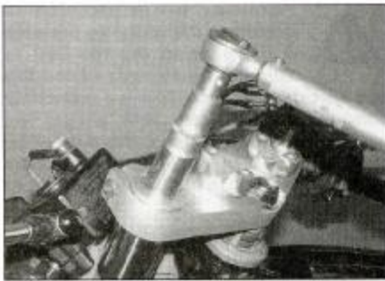
6.9 If slackened, tighten the fork top bolt to the specified torque
