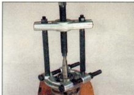
5.3 This bearing puller clamps behind the bearing and pressure is applied to the shaft end to draw the bearing off
