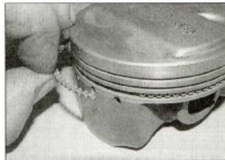
17.10a Install the oil ring expander in its groove ...
