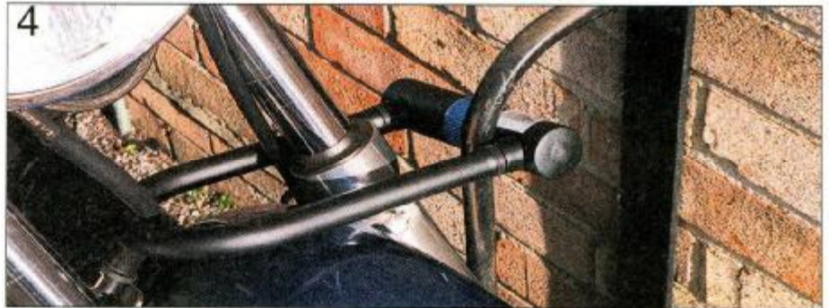
4 U-locks can be used to secure the bike to a solid object – ensure you purchase one which is long enough
