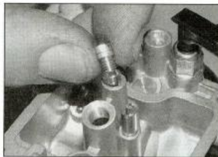
10.13 . . . and the starter jet with its collar
