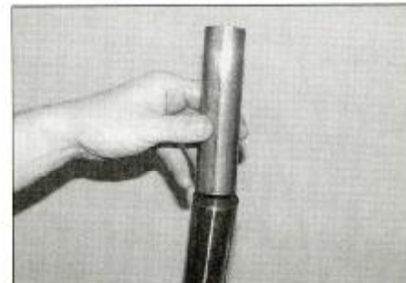
7.4a Remove the spacer ...
