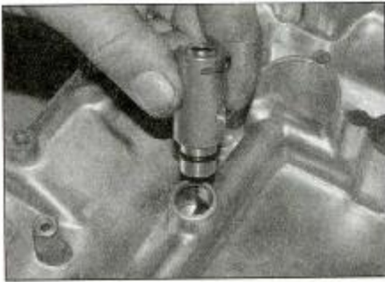
24.5a Pull the relief valves out of the sump . . .
