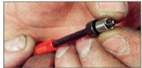
2.28 ... fit insert on the installing tool ...
