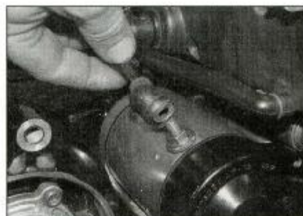
28.7 Connect the lead and secure it with the nut
