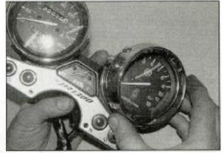
16.7b ... and remove the rims ...
