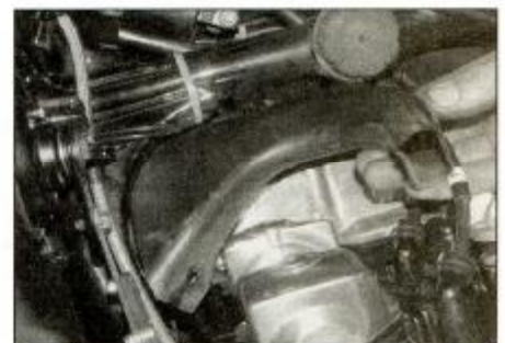
5.6c . . . and remove the air ducts
