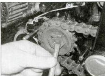
16.9a Bend down the lockwasher tabs ...
