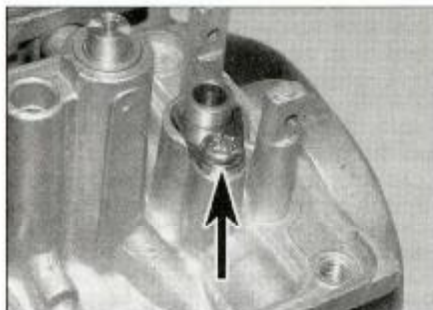
8.8 Undo the screw (arrowed) and remove the plate, then withdraw the seat
