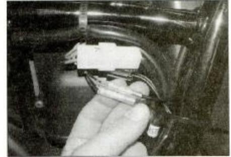
7.2c Carburettor heater wiring connectors – 2002-on models
