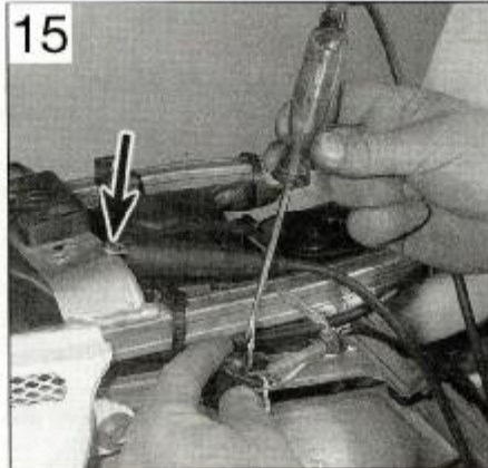
15 . . . or a test light - note the earth connection to the frame (arrow)
