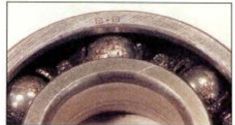
5.18 Example of ball journal bearing with damaged balls and cages
