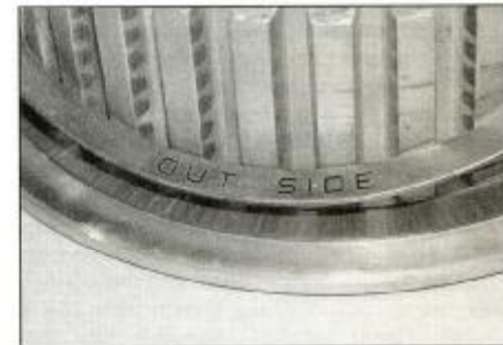
18.21b ... followed by the anti-judder spring, with the OUTSIDE mark facing out
