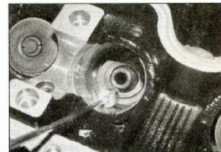
14.7b ... then remove the spring seat
