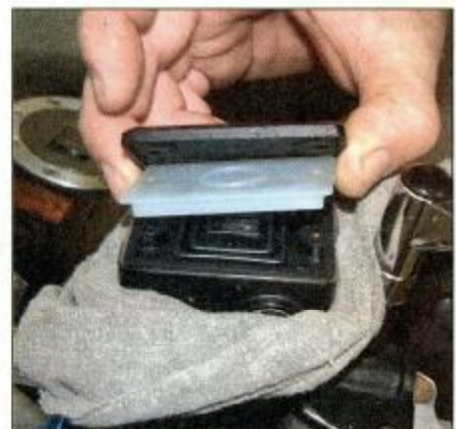
4 Ensure that the diaphragm is correctly seated before installing the plate and cover. Tighten the cover screws securely.
