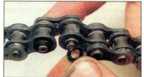
8.5 . . . install the O-rings over the pin ends . . .
