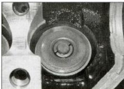
14.31c Check that the collets are correctly seated . . .
