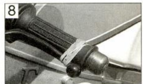
Hold clutch lever back against the handlebar with elastic bands or a cable tie
