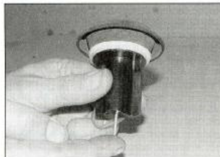
8.17b . . . then push the needle up and withdraw it
