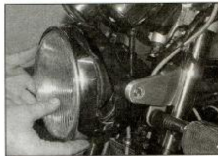
7.1b . . . and draw the rim out of the shell as described
