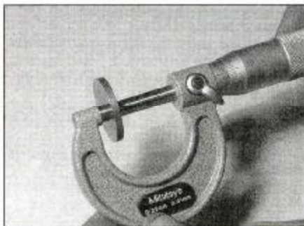
Tappet shims are measured with a micrometer
