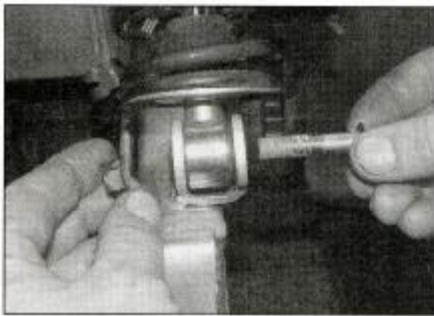
11.3a Unscrew the nut and withdraw the bolt ...
