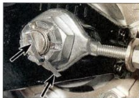
2.5 Bend split pin (cotter pin) arms as shown (arrows) to secure a castellated nut
