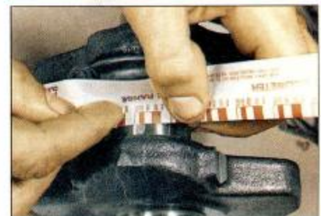
3.16 Measuring the width of the crushed Plastigauge
