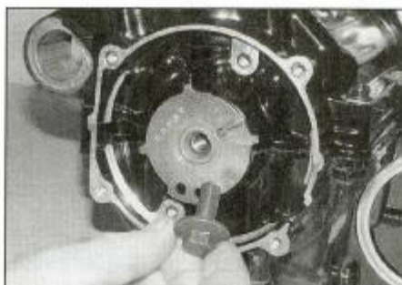
25.24c ... then install the bolt and tighten it to the specified torque
