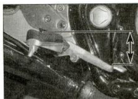
9.7a Measure the distance between the top of the footrest and the top of the brake pedal as shown
