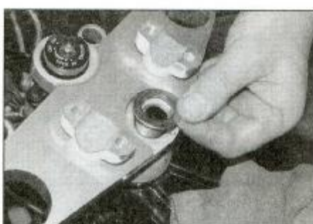
9.17a Fit the washer (where applicable) ...
