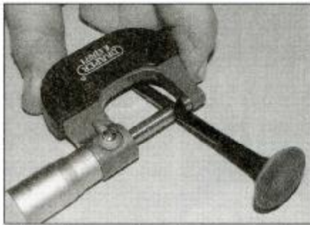
14.15a Measure the valve stem diameter with a micrometer
