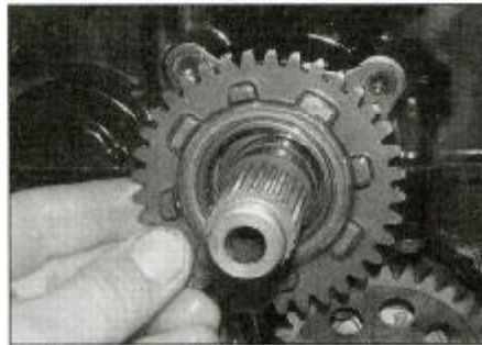
18.22c ... and the oil pump drive gear onto the shaft
