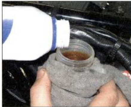
8 Top up with new clean DOT 4 hydraulic fluid, until the level is above the line. Take care to avoid spills (see Warning above). Do not overfill.
