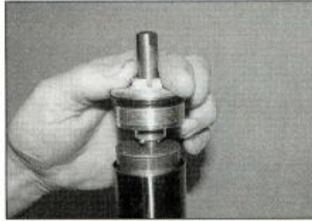
7.8 Fit a new O-ring onto the top bolt then thread it into the fork tube
