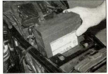
3.3b . . . and lift the battery out of its box
