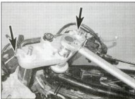
19.14c . . . then tighten the nut to the specified torque setting, followed by the clamp bolts (arrowed)
