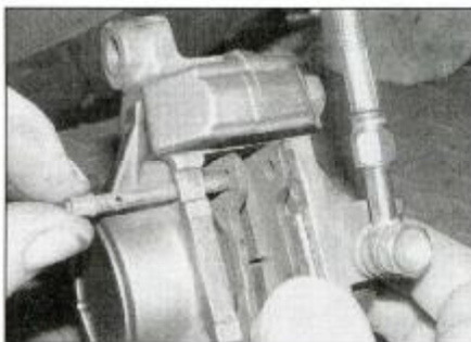
2.19b . . . and insert one of the pins
