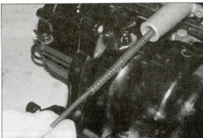
9.10a Install the springs ...
