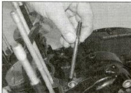
10.10b . . . and withdraw the spring and rod
