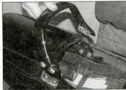
4.2b . . . and remove the grab-rail
