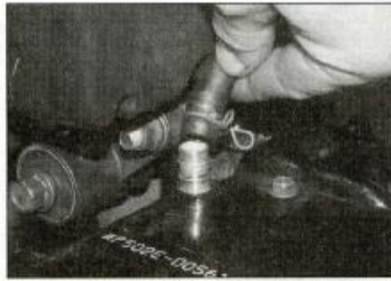
5.11a Detach the crankcase breather hose ...
