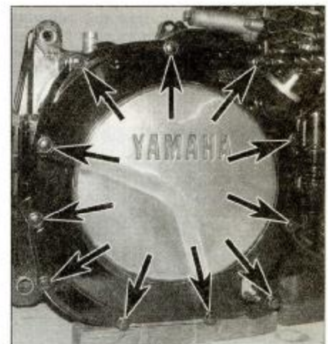
18.2 Unscrew the bolts (arrowed) and remove the cover
