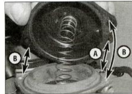
10.21c Fit the top cover, aligning the air passage with the O-ring (A) and the peg with the hole (B)
