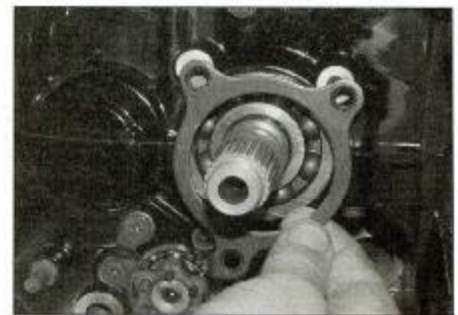
25.23 Use a threadlock on the retainer plate screws
