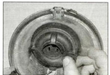
7.3a Remove the dust cover
