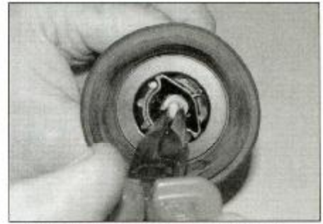
8.17a Remove the jet needle holder . . .
