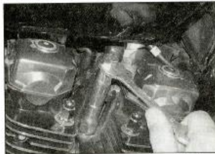
2.4 Unscrewing the spark plug using the Yamaha tool
