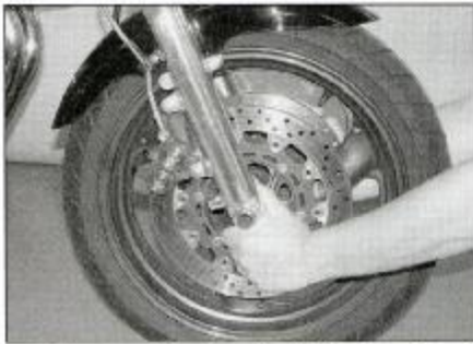
19.4 Checking for play in the steering head bearings
