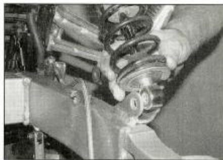
11.3b ... then pivot the shock back
