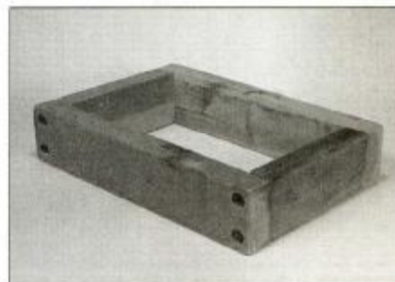
6.4 An engine support made from pieces of 2 x 4 inch wood
