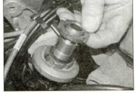
9.9b ... then unscrew the locknut ...
