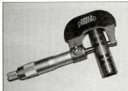
16.12b Measure the external diameter of the pin ...
