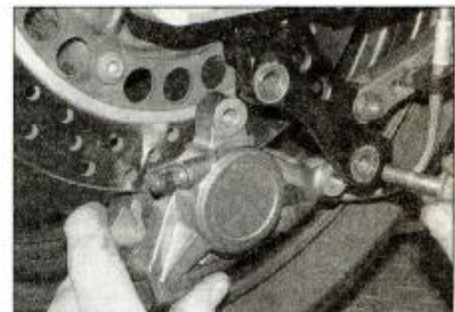
5.15 Slide the caliper onto the disc and install the bolts
