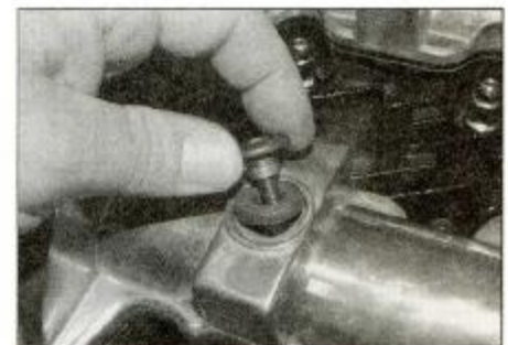
8.9b Fit the bolts with their washers
