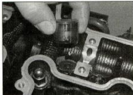
11.23 Fit the shim into the follower, then fit the follower into its bore and onto the valve
