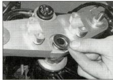
19.14a Install the washer (1997-on models) . . .
