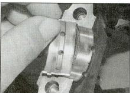
29.5 To remove a main bearing shell, push it sideways and lift it out
