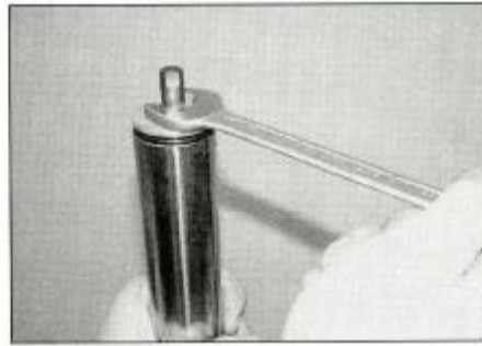
7.3a Thread the top bolt out of the tube
