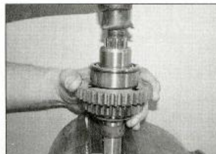
32.30c ... then drive the bush onto the shaft as shown ...
