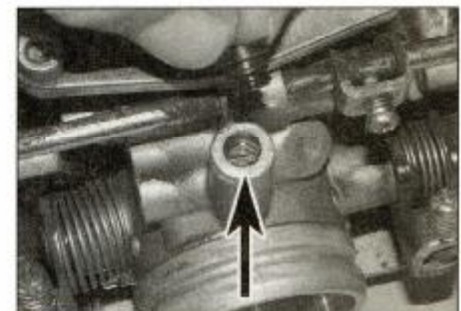
8.12 Remove the blanking cap to access the pilot screw (arrowed)
