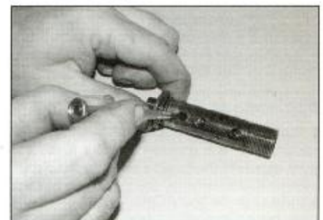
20.4 Check the bypass valve action as described
