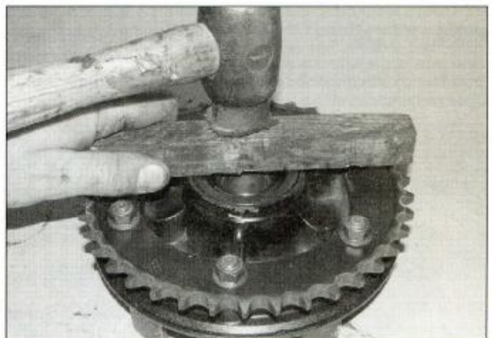
14.31b Using a piece of wood as shown automatically sets the seal flush
