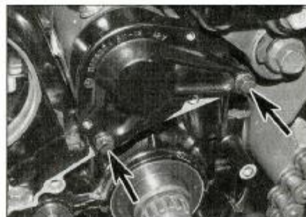
28.3a Unscrew the bolts (arrowed) . . .
