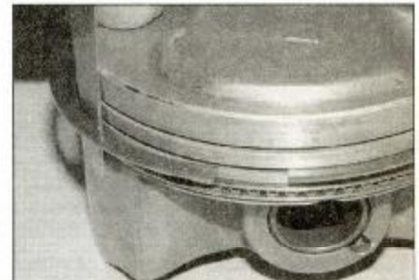
17.12b Old pieces of feeler gauge blade can be used to guide the ring over the piston
