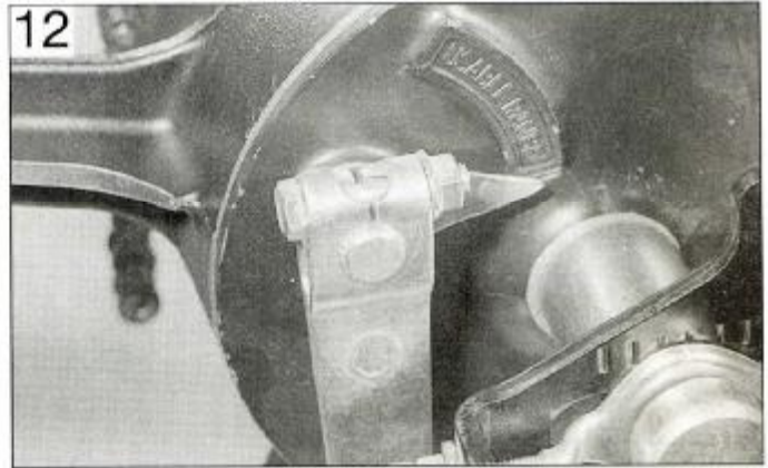
12 On drum brakes, check the angle of the operating lever with the brake fully applied. Most drum brakes have a wear indicator pointer and scale.
