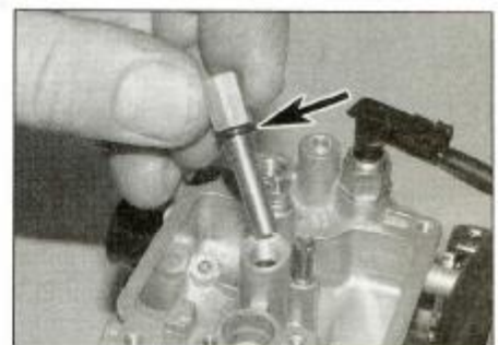
10.14a Fit a new O-ring (arrowed) then install the emulsion tube
