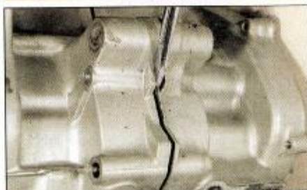
7.1 If a pry point is provided, apply gently pressure with a flat-bladed screwdriver
