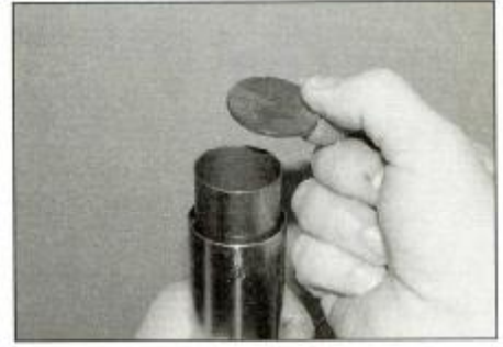
7.3b On XJR1300 models remove the adjuster plate
