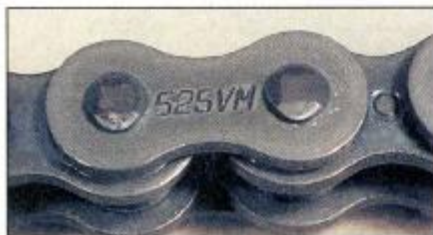
8.10 Typical chain size and type marking
