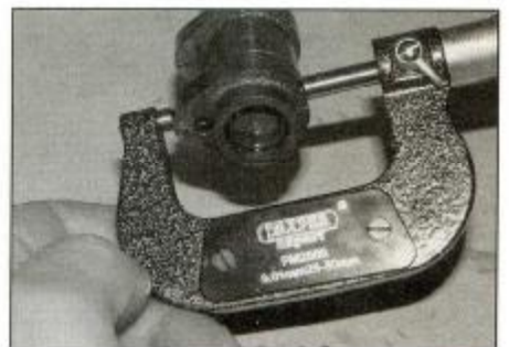
11.13 Measure the height of the camshaft lobes with a micrometer
