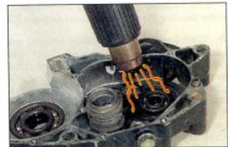
5.13 Using a localised heat source to aid bearing removal
