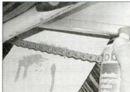
1.16 Apply the lubricant to the overlap between the sideplates. Note the use of a piece of card to prevent lubricant contacting the tyre
