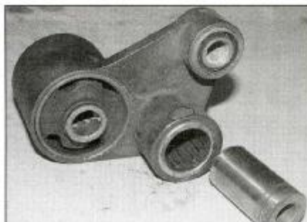
5.25b Note the spacer and bearing in the upper frame bolt bore
