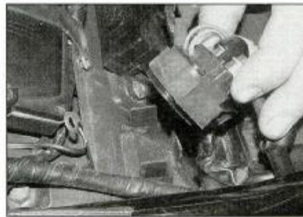
27.7c Lift the relay off its mounts
