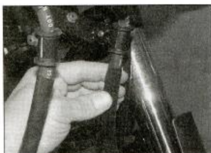
9.3 Flex the brake hose and check for cracks, bulges and leaking fluid
