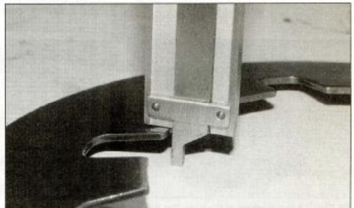
18.14 Measure the free height of the spring as shown
