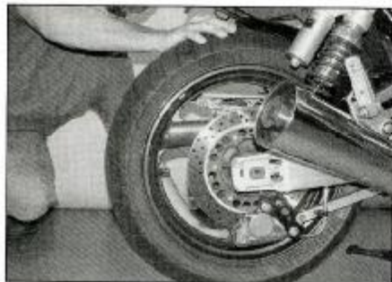
13.2 Checking for play in the wheel bearings
