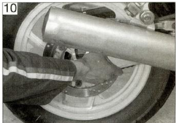
10 Grasp the swingarm at the ends to check for play in its pivot bearings
