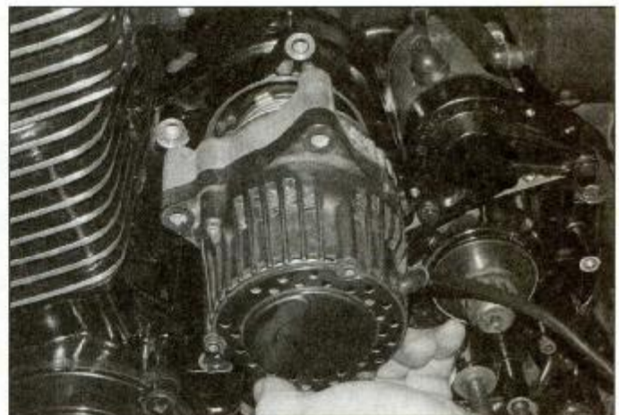
32.9b . . . and remove the alternator
