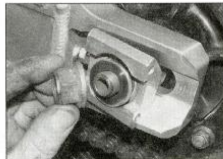
13.13c ... the washer and the nut
