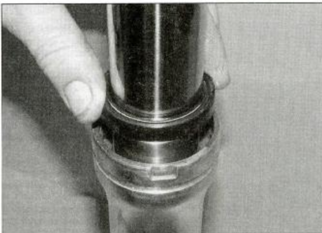
8.22a Smear the new oil seal with clean fork oil then slide it down the tube
