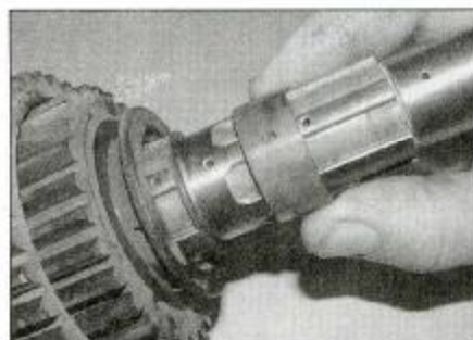
32.30b ... and the 3rd gear pinion bush ...
