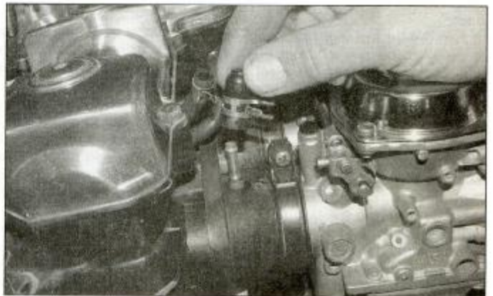
4.4a Remove the blanking caps . . .
