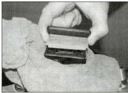
6.25 Make sure the diaphragm is correctly seated before fitting the plate and cover
