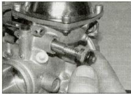
8.31e . . . and withdraw the plunger assembly
