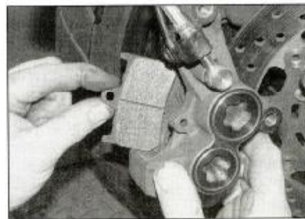
2.3d Lift the pads out of the caliper ...
