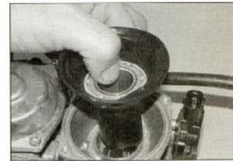
8.3 Carefully withdraw the diaphragm/piston assembly
