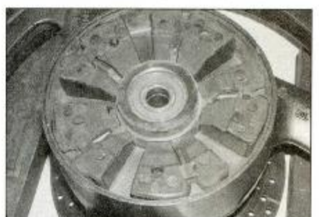
17.3 Check the rubber dampers
