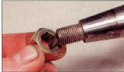
2.23 A thread repair tool being used to correct an external thread
