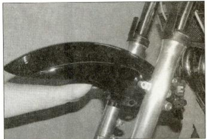
5.2b . . . and remove the mudguard
