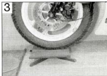
Front wheel mounted on a surface plate for steering head bearing lower race check
