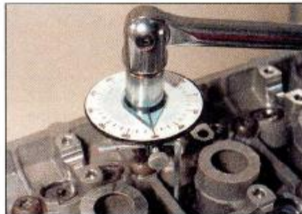
4.2 Angle tightening can be accomplished with a torque-angle gauge ...
