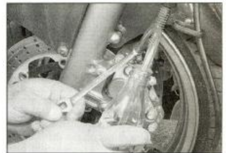
9.5c To bleed the brakes, you need a spanner, a short section of clear tubing, and a clear container half-filled with brake fluid
