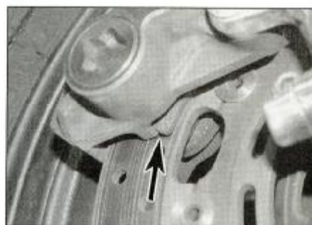
8.2b Front brake pad wear indicator (arrowed)
