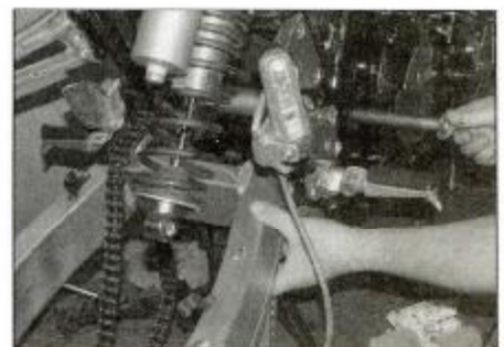
13.13a Locate the swingarm in the frame, looping the chain around the front then slide the pivot bolt through . . .
