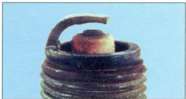
Worn plug – Worn electrodes will cause poor starting in damp or cold conditions and will also waste fuel.
