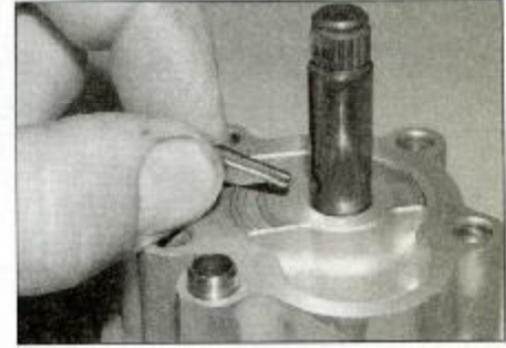
23.15h Fit the drive pin ...
