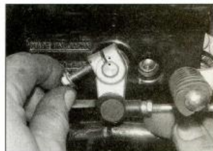
22.2 Unscrew the bolt and slide the arm off the shaft, noting the alignment punch marks
