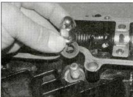
12.10a Install the nuts with their washers . . .
