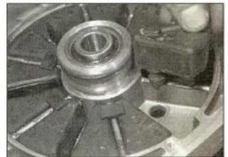
Cush drive rubbers dampen out transmission shocks
