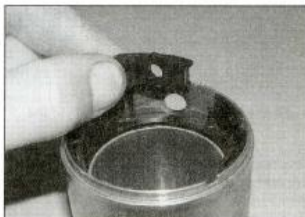
29.16b ... and the insulator
