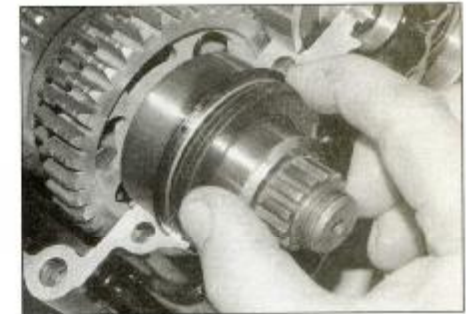
25.14a Fit a new output shaft oil seal
