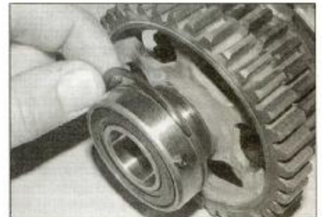
31.2b . . . and remove the half-ring retainer
