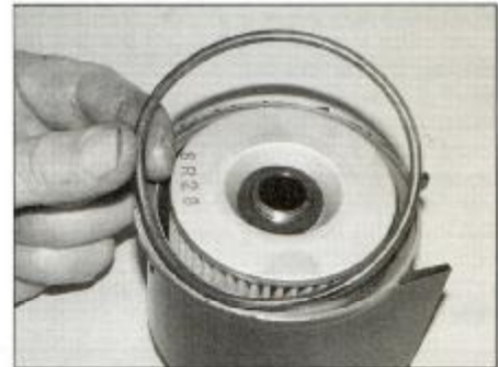
20.6a Fit the greased O-ring into the groove ...
