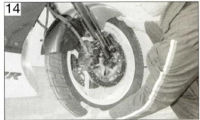
14 Check for wheel bearing play by trying to move the wheel about the axle (spindle)
