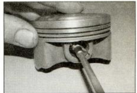
16.12c ... and the internal diameter of the bore in the piston
