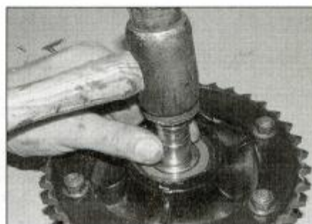
14.26 Remove the spacer from inside the coupling
