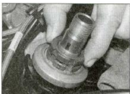
9.16 Tighten the locknut as described so the notches align
