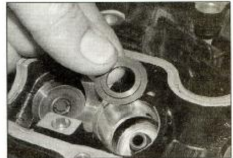
14.27 Lay the spring seat over the top of the guide and onto the head
