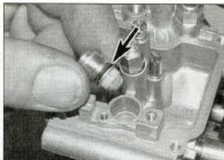
10.15a Fit a new O-ring (arrowed) then install the seat . . .
