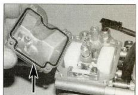
10.18 Fit a new seal (arrowed) then install the float chamber
