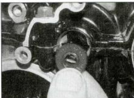
20.8 Fit a new pushrod oil seal if necessary
