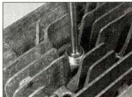
Installing a Helicoil thread insert in a cylinder head
