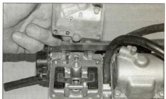
10.7b . . . then install the float chamber
