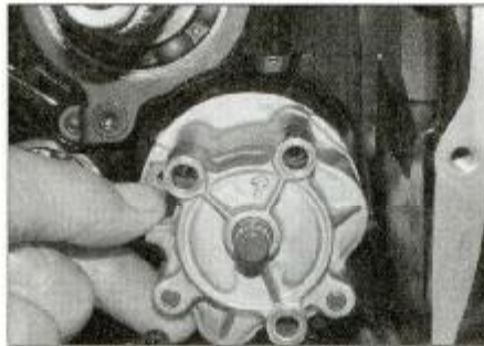
23.19 Install the pump, aligning the arrow with that on the crankcase
