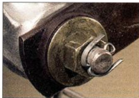
2.6 Bend split pin (cotter pin) arms as shown to secure a plain nut
