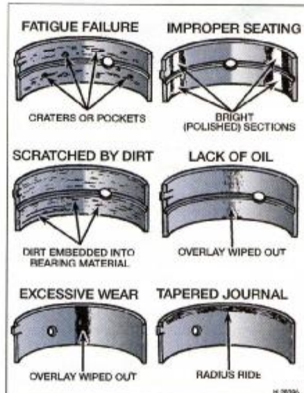
5.17 Typical bearing failures
