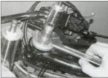
19.12 If the tool is not available, adjust the bearings as described – here a C-spanner is being used
