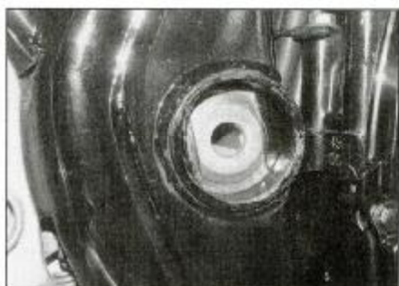
13.13b . . . locating the flats in the cutout
