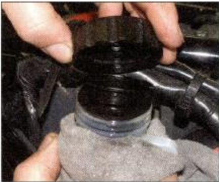
7 Unscrew the reservoir cap and remove the diaphragm plate and the diaphragm.
