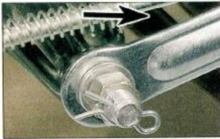
2.7 Correct fitting of R-pin. Arrow indicates forward direction
