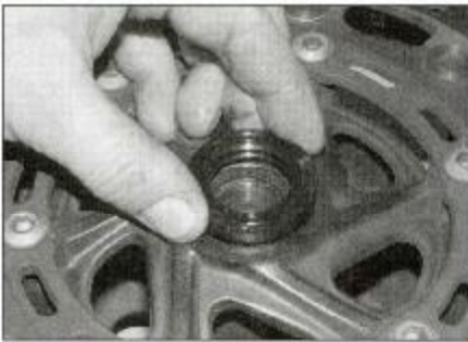
14.12a Press or drive the seal into place
