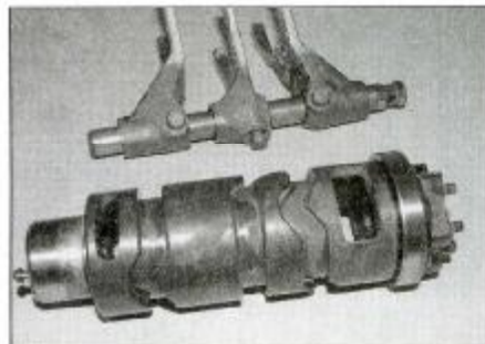
33.9 Check the fork guide pins and the grooves in the selector drum
