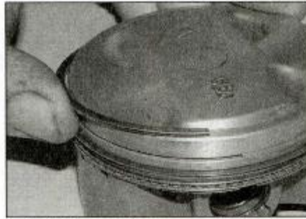
16.4 Remove the rings carefully - they break easily
