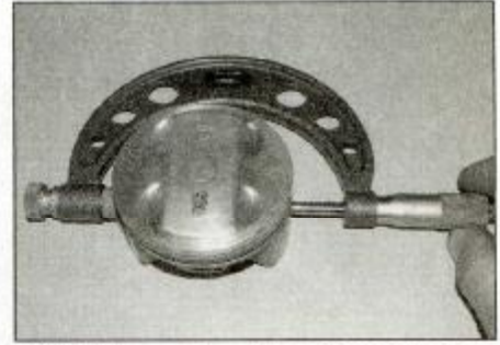
16.11 Measure the piston diameter with a micrometer at the specified distance from the bottom of the skirt
