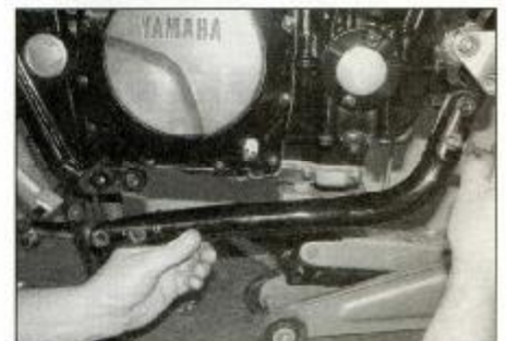
5.22 Unscrew the four bolts and remove the frame cradle section
