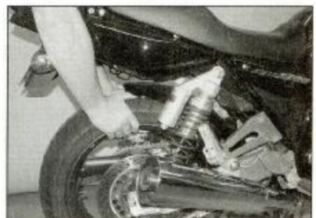
18.7b Checking for play in the suspension mountings and swingarm bearings
