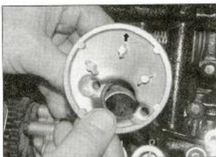
24.10b . . . then install the strainer body with the arrow to the front
