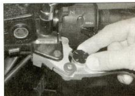
10.5 Adjusting the clutch lever span
