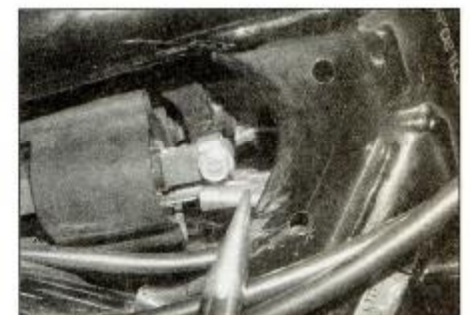
3.4a Disconnect the primary circuit connectors from the coil
