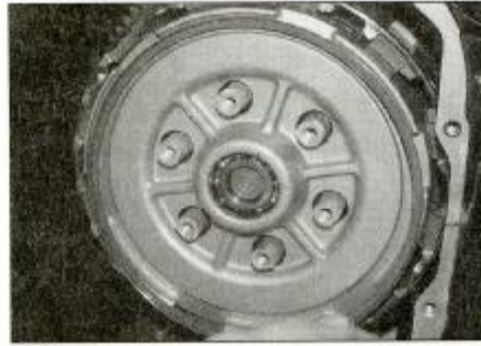
18.28c Fit the spring seat ...
