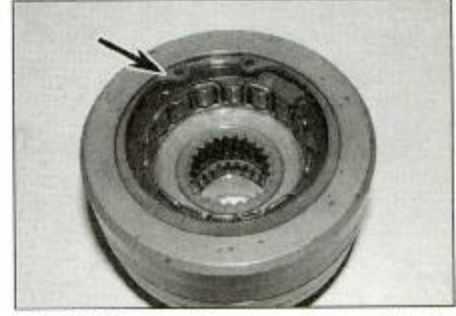
28.13b Remove the circlip (arrowed) and lift the sprag assembly out
