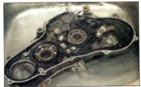
5.12 A casing can be immersed in a sink of boiling water to aid bearing removal
