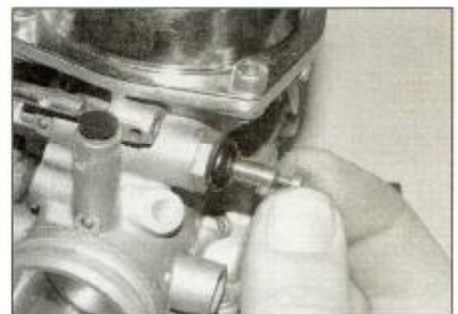
8.31c Check the action of the plunger as described
