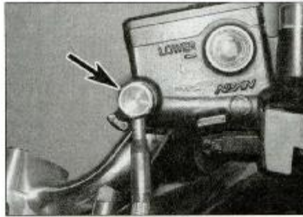
19.6 Clutch hose banjo bolt (arrowed)
