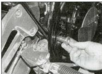
13.8a Withdraw the pivot bolt ...
