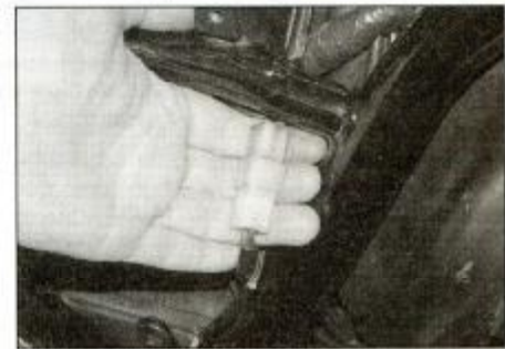
5.13 Disconnect the alternator wiring connector
