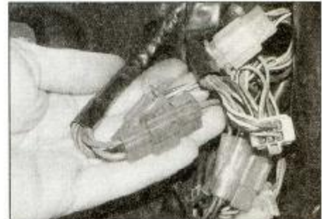
18.2 Disconnect the ignition switch wiring connectors
