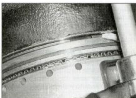
15.25 Carefully compress and feed the rings in using a screwdriver and/or fingernails
