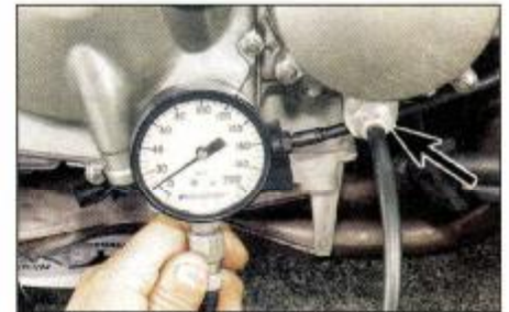
3.21 Oil pressure gauge and take-off point adapter (arrow)
