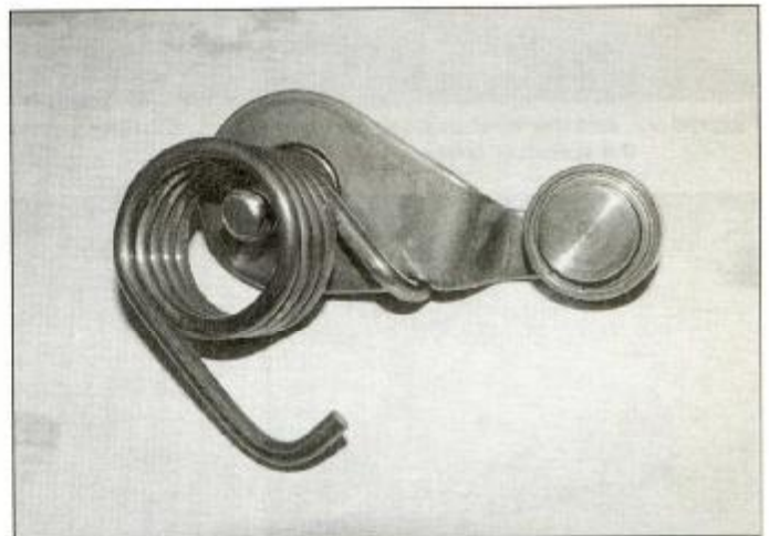
22.8b ... and the stopper arm assembly as described
