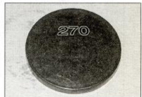
23.16 Size marking is stamped on one side of the shim
