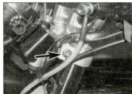
6.4 Slacken the clamp bolt (arrowed) in the top yoke
