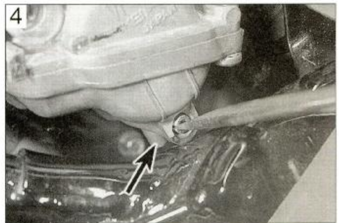
Connect a hose to the carburettor float chamber drain stub (arrow) and unscrew the drain screw
