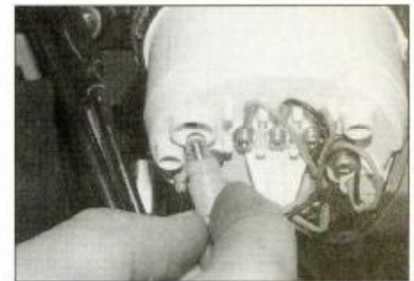
17.3a Pull out the bulbholder ...
