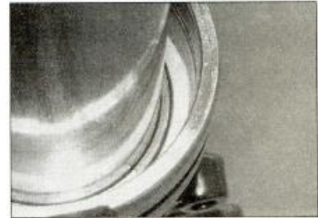
8.21 Remove the washer and check the bush is fully home
