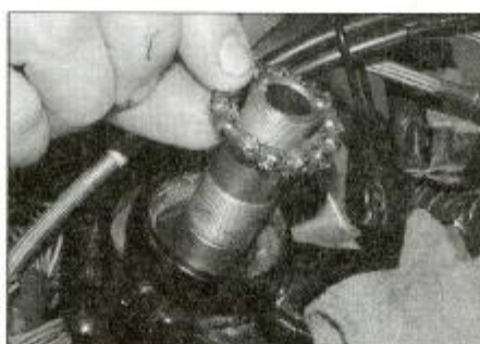
9.15a Fit the upper bearing ...
