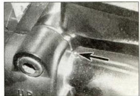
5.3b . . . noting how the clamp surfaces align with the punch mark (arrowed)
