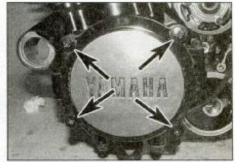
4.7 Undo the screws (arrowed) and remove the cover and gasket
