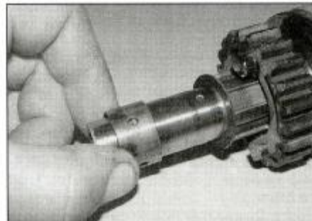
32.18b ... and the 5th gear pinion bush ...
