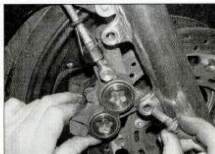
4.15 Slide the caliper onto the disc and install the bolts
