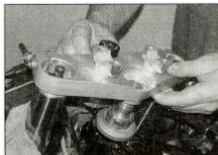
18.10 Ease the yoke up off the steering stem and forks
