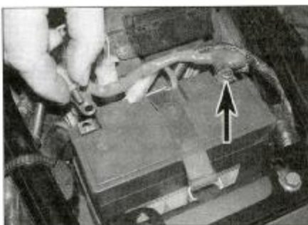
3.2 Disconnect the negative terminal first, then the positive (arrowed)
