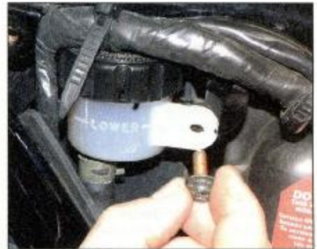
9 Ensure that the diaphragm is correctly seated before installing the plate and cap. Tighten the cap securely. Remount the reservoir.
