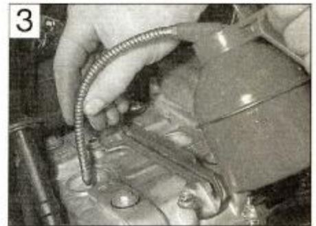
Bores can be temporarily sealed with a squirt of motor oil
