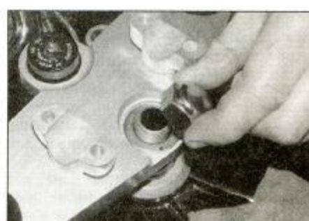
9.17b ... and the steering stem nut ...
