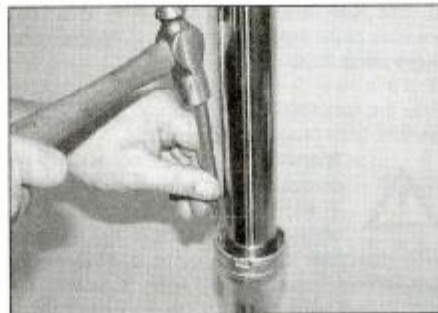
8.20c A drift can be used to tap the bush into place
