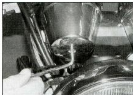
17.2a Unscrew the cover screw ...
