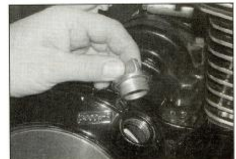
7.3 Remove the oil filler cap from the clutch cover
