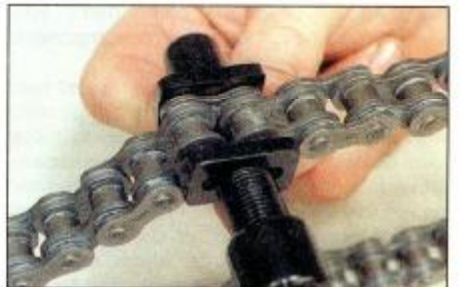
8.7 Push the sideplate into position using a clamp
