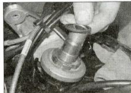
9.9c ... and remove the rubber washer
