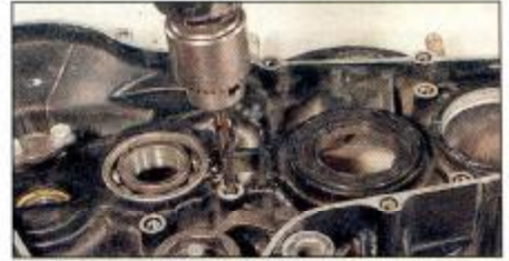
2.26 To install a thread insert, first drill out the original thread ...
