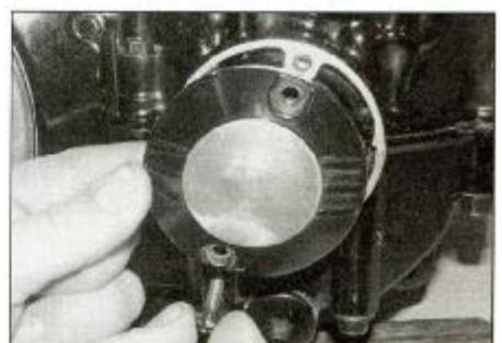
25.25 Install the crankshaft end cover
