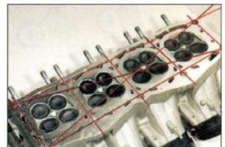
3.23 Check for warpage in these directions
