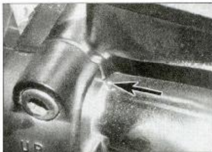
19.19 Align the clamp mating surfaces with the punch mark (arrowed)
