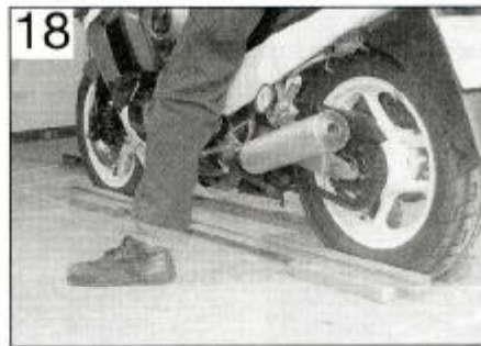
Two straightedges are used to check wheel alignment
