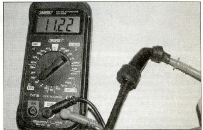
3.6 Measuring the resistance of the spark plug cap
