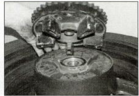
14.14 Removing the sprocket coupling
