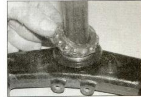
9.14c ... then fit the bearing
