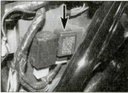
11.3 Turn signal relay (arrowed)
