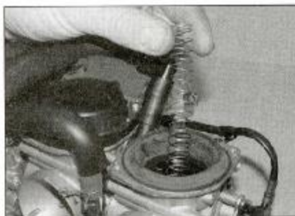
10.21b . . . then insert the spring
