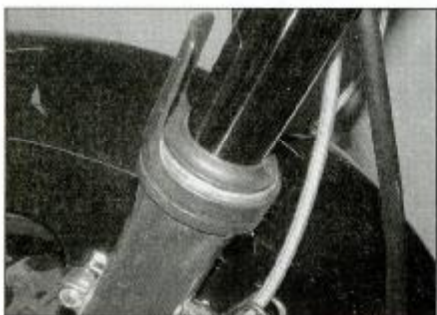
18.3 Check for oil leakage, scratches, corrosion, and pitting on the fork tube
