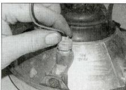
7.10a Draw out the bulbholder ...
