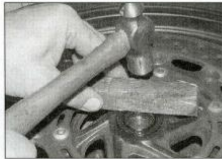
14.12b Using a piece of wood as shown automatically sets the seal flush
