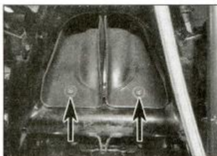
5.6a Undo the screws (arrowed) . . .
