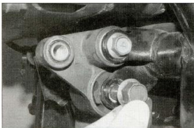
5.27a If required, unscrew the bolts . . .
