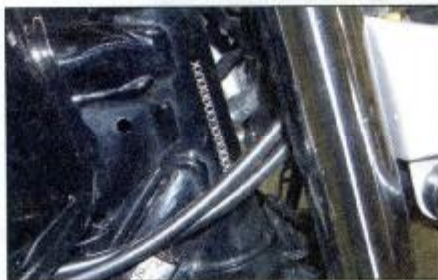
The frame number is stamped into the right-hand side of the steering head
