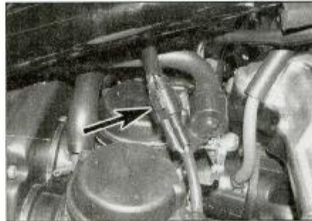
7.2b Throttle position sensor wiring connector (arrowed) – 2002-on models
