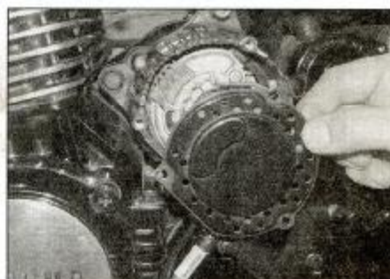
24.1b . . . and remove the alternator cover
