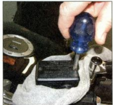
2 If the level is below the LOWER line, undo the two reservoir cover screws and remove the cover, diaphragm plate and diaphragm.
