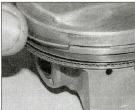
17.13 Finally fit the top ring
