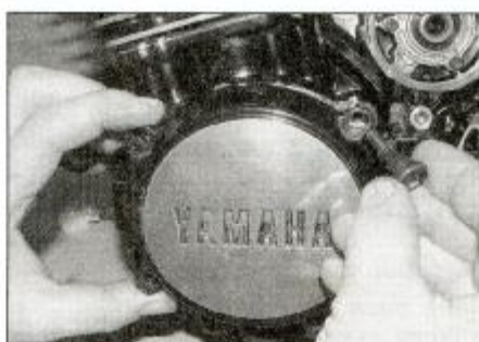
23.21b . . . and install the cover
