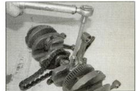
30.27 ... and tighten them as described, first to the initial torque, then to the final torque
