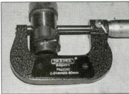
11.18 Measure the cam bearing journals with a micrometer
