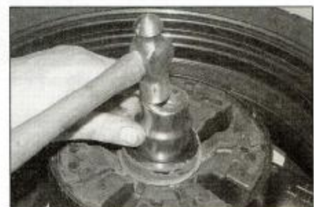
14.21 A socket can be used to drive in the bearing
