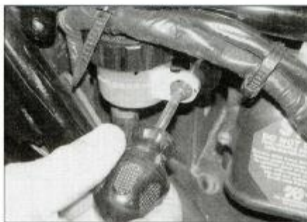
7.3b Undo the screw and displace the reservoir . . .
