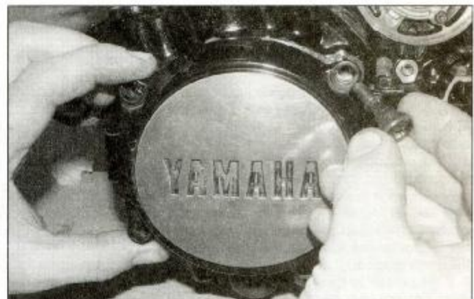
4.10b . . . and install the cover
