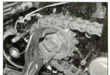
16.13 Bend the lockwasher tabs up against the nut
