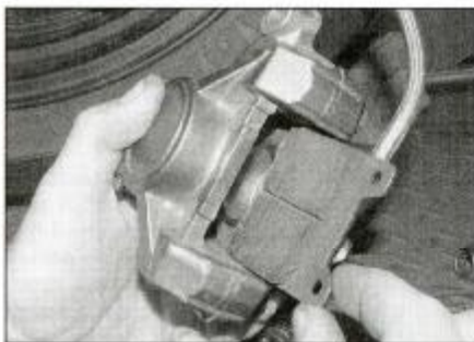
2.17d . . . and lift the pads out of the caliper
