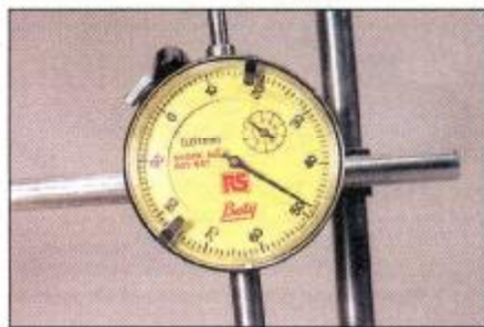
3.17 Dial gauge reading of 1.48 mm
