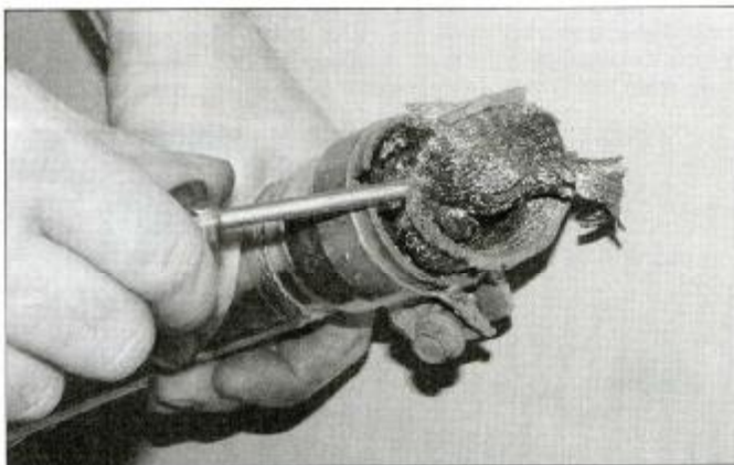
14.3a You will probably have to dig the old sealing ring out
