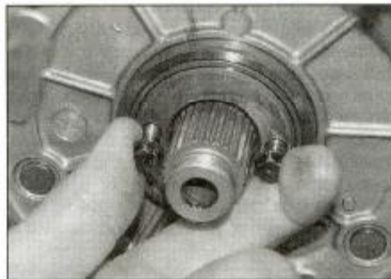
18.9 Use a pair of bolts as described to draw the collar out
