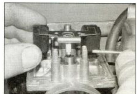
10.5b . . . then install the float assembly and pin
