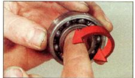
5.19 Hold outer race and listen to inner race when spun
