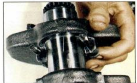
3.15 Plastigauge placed across shaft journal
