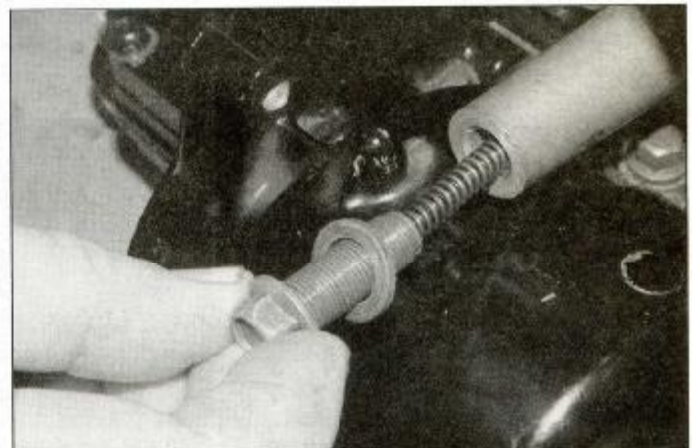
9.10b ... then fit the cap bolt with its washer
