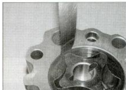
23.11 Measuring outer rotor to cover or body clearance
