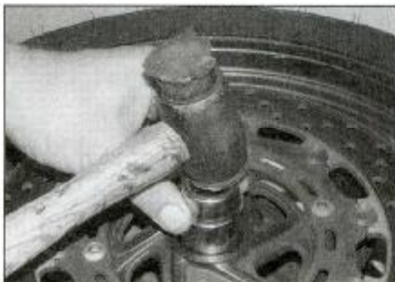
14.9 A socket can be used to drive in the bearing
