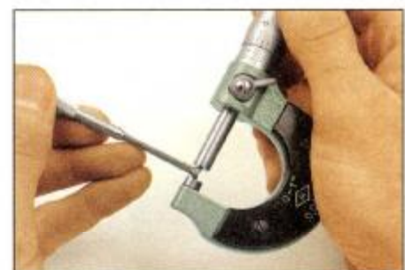
3.10 . . . then measure the gauge with a micrometer
