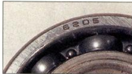
5.16 Typical bearing marking
