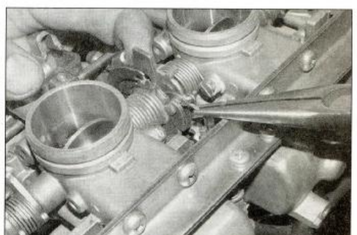
11.5b ... then the decelerator cable
