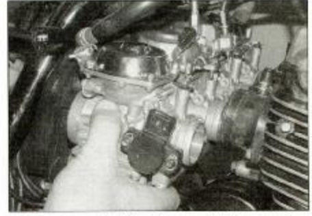
7.7c ... and slide them out to the right-hand side of the bike
