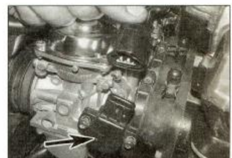
7.3a Throttle position sensor (arrowed) with wiring connector disconnected – 1995 to 2001 models
