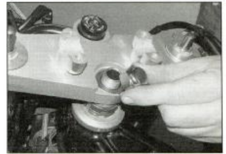
19.14b . . . and the steering stem nut . . .
