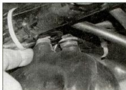
5.6b . . . release the pegs from the grommets . . .
