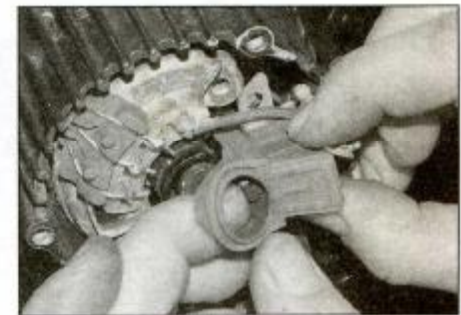
32.2c Push the brushes in and check they move freely
