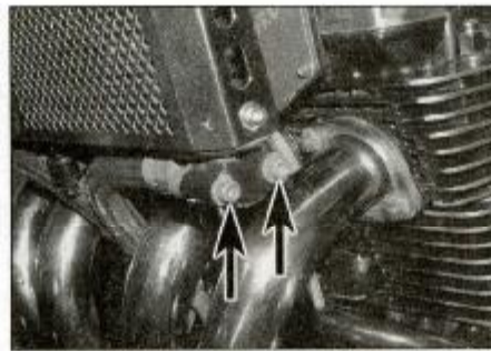
7.2a Unscrew the bolts (arrowed) on each side and detach the hoses from the cooler
