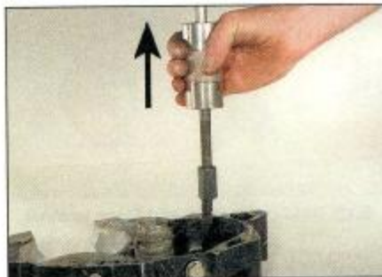
5.7 . . . attach the slide hammer to the bearing puller
