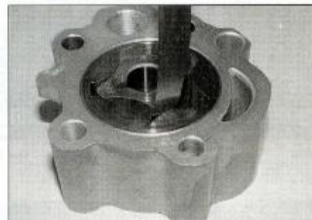
23.12 Measuring inner rotor tip to outer rotor clearance
