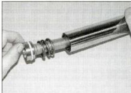
8.18a Slide the damper rod into the tube and all the way down so that it projects from the bottom
