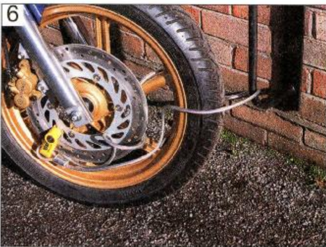
6 A disc lock combined with a security cable provides additional protection
