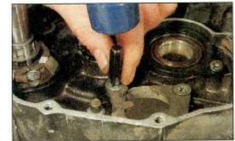
2.13 A sharp tap on the head of a fastener will often break free a corroded thread
