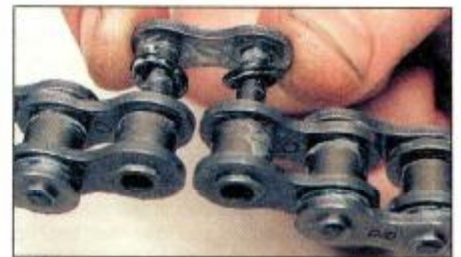
8.4 Insert the new soft link, with O-rings, through the chain ends . . .
