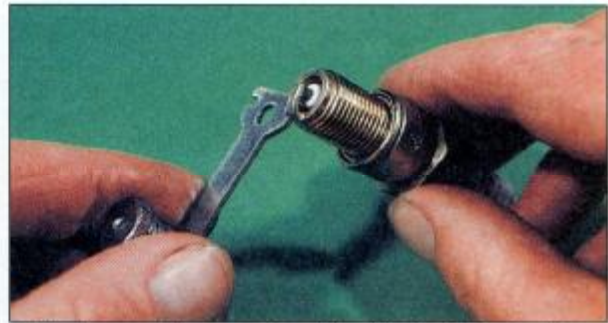
Electrode gap adjustment – bend the side electrode using the correct tool.
