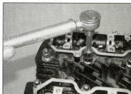
12.10b . . . and tighten them as described to the specified torque setting
