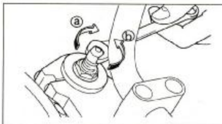
12.2a Adjusting fork pre-load – A to increase, B to decrease
