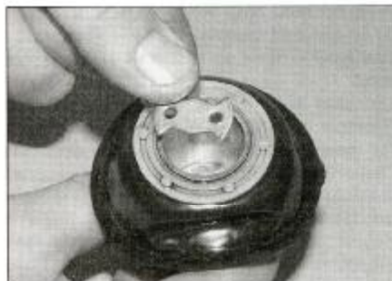
10.8f Fit the retainer plate . . .
