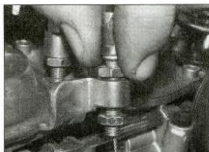
16.6b Slacken the top nut, move the cable down in the bracket and adjust the position of the bottom nut as required
