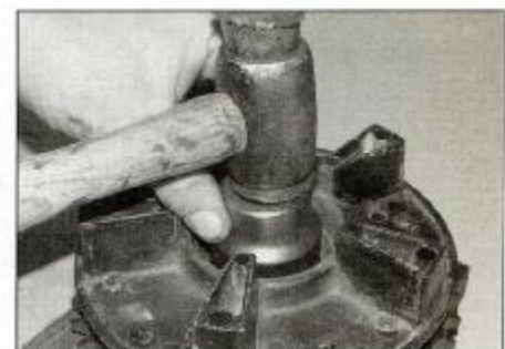
14.27 A socket can be used to drive the bearing out . . .
