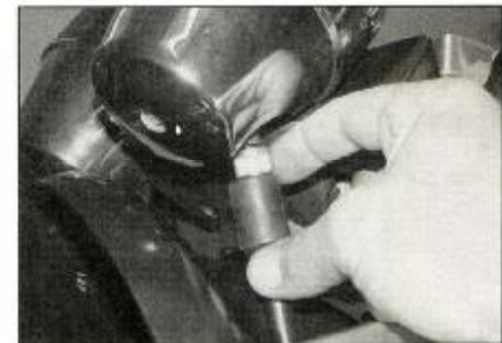
16.11 ... and from the speedometer, and withdraw it
