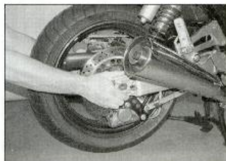
18.7a Checking for play in the swingarm bearings
