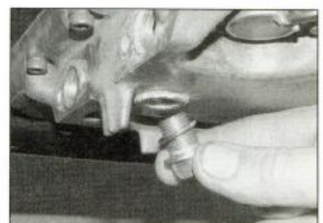
7.5 Install the drain plug using a new sealing washer
