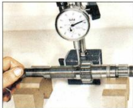
3.18 Using a dial gauge to measure shaft runout
