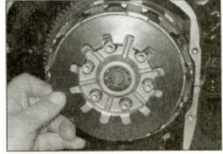
18.28d ... the diaphragm spring ...
