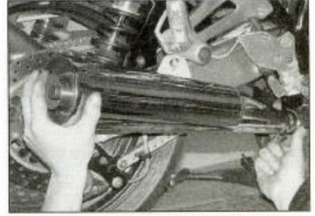
14.2b . . . and remove the silencer
