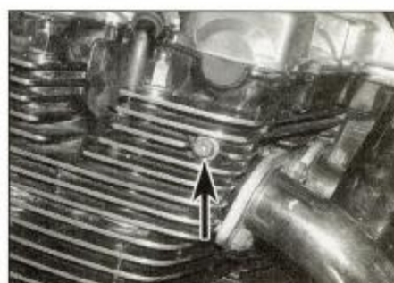
30.9 Oil gallery check bolt (arrowed)
