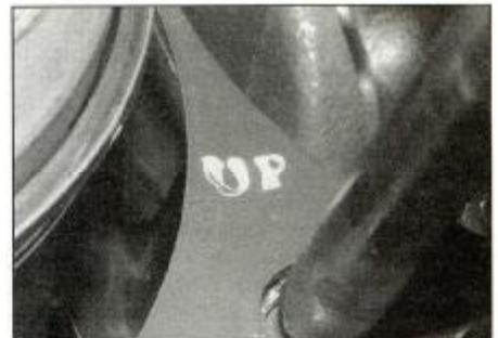
15.22b ... making sure the UP mark reads correctly
