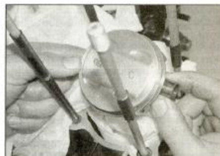
16.3b . . . then push out the pin and remove the piston
