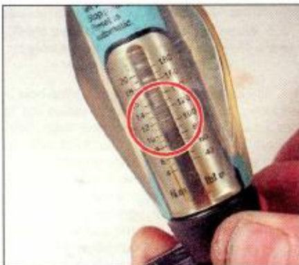
4.1 Set the torque wrench index mark to the setting required, in this case 12 Nm
