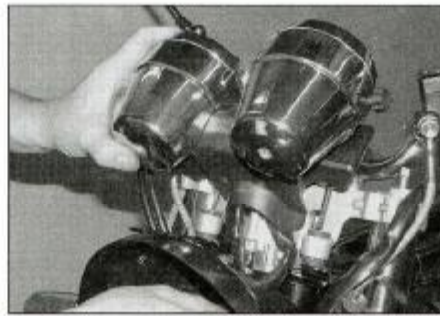
15.4b . . . then lift the cluster away, feeding the wiring out of the headlight as you do
