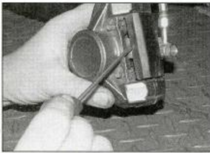
2.17a Remove the pad cover
