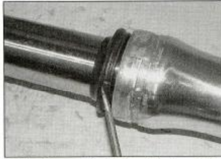
8.7b Prise out the dust seal using a flat-bladed screwdriver
