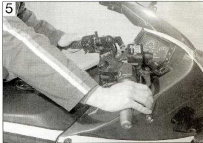
Hold the front brake on and pump the front forks up and down to check operation
