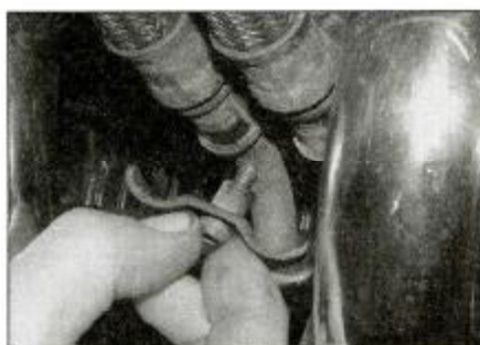
7.3a Unscrew the bolt and remove the pipe holder
