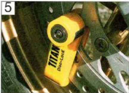
5 A typical disc lock attached through one of the holes in the disc
