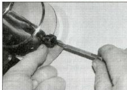
16.3 Undo the screw and remove the knob
