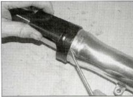
8.7a Where fitted, remove the protector
