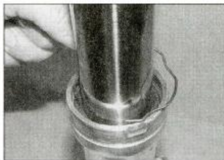
8.23 Install the retaining clip . . .
