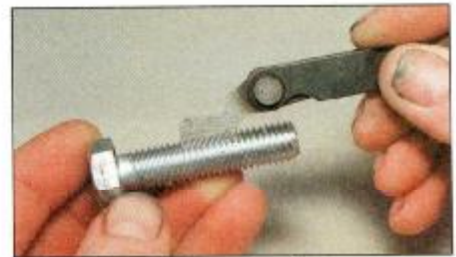
2.12 Using a thread gauge to measure pitch
