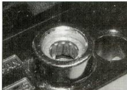
22.11e . . . and check the bearing
