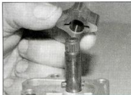
23.15i ... then locate the inner rotor onto it ...
