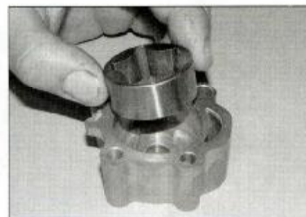
23.15a Fit the outer rotor . . .
