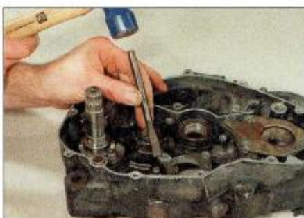
2.16 Using a hammer and chisel to free a seized fastener
