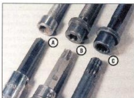
2.1 Internal hexagon/Allen (A), Torx (B) and splined (C) fasteners, with corresponding bits
