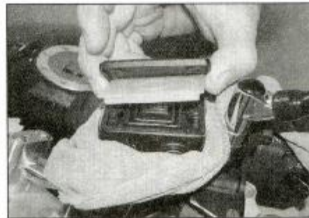
19.24 Make sure the diaphragm is correctly seated before installing the plate and cover
