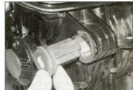
5.26b Remove the damping rubbers if loose
