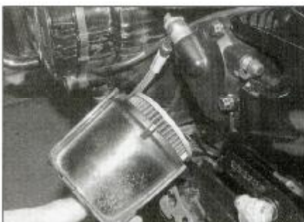
20.3b . . . and remove the filter assembly
