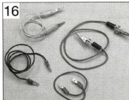
16 A selection of jumper wires for making earth (ground) checks
