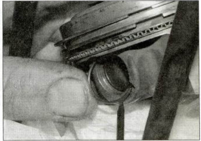
16.16b Do not over-compress the circlip and make sure it seats in the groove
