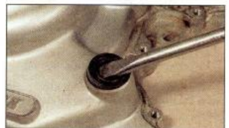
6.1 Prise out oil seals with a large flat-bladed screwdriver
