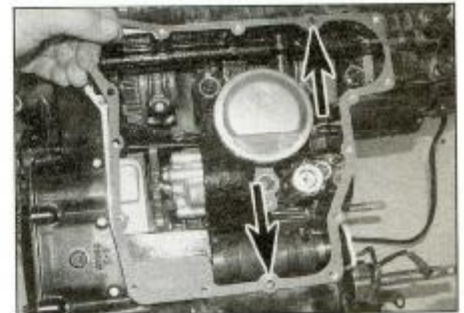
24.11 Fit the dowels (arrowed) and a new gasket . . .
