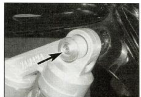
11.4 Unscrew the upper mounting bolt and remove the shock
