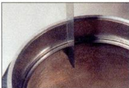
3.1 Feeler gauges are used for measuring small gaps and clearances - thickness is marked on one face of gauge
