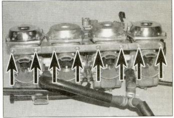
9.6a Upper bracket screws (arrowed)
