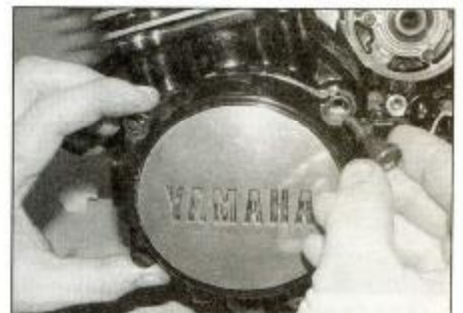
11.33b . . . and install the cover
