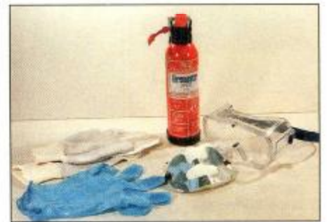
1.6 A fire extinguisher, goggles, mask and protective gloves should be at hand in the workshop
