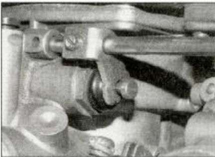
8.31g Make sure the arms locate correctly on the plungers . . .
