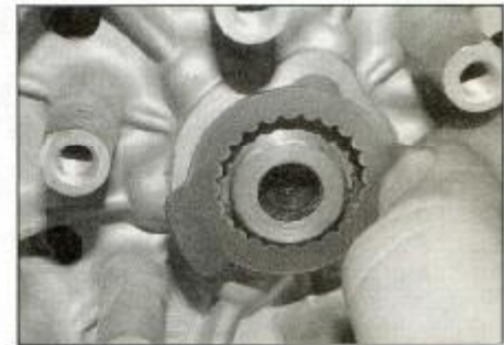
18.25b ... then fit the new lockwasher ...
