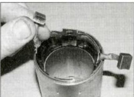
29.16c Locate the brush assembly ...
