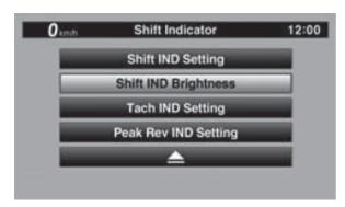
Select "Shift IND Brightness", then use the wheel switch to adjust the setting. Short push the wheel switch to confirm the setting and exit.
