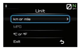
This module allows you to change the measurement units. Each of the three items contain a sub-menu where the desired unit is selected.
