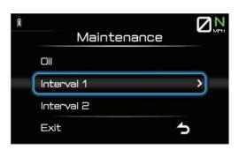
This module allows you to record distance traveled between engine oil changes "Oil", and two other maintenance intervals of your choice "Interval 1"/ "Interval 2". Short press the "MENU \$\int "
