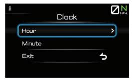
This module allows you to set the 12-hour clock. The hours and minutes are set individually. "All Reset"
