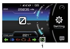
1. Transmission gear display (Relocated)
