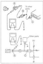
If continuity is indicated, the circuit is shorted to the ground between terminals (A) and (B).
