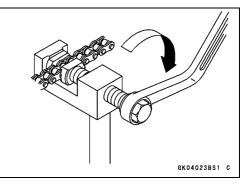
• Set the plate holder (B) [A] and cutting and riveting pin [B] as shown in the figure.
