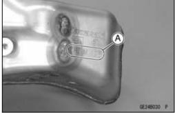
Premuffler Chamber Mark Position [A]
