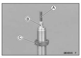
• Using rod guide case wrench [A], remove the piston rod guide case from the inner tube.
