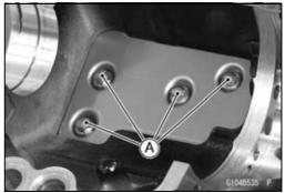
• Press and insert the fitting [A] in the upper crankcase [B] until it is bottomed.
