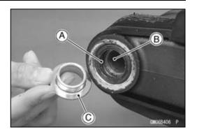
• Screw the adjusting collar [A] into the frame [B] so that the collar does not project the swingarm mating surface [C].
