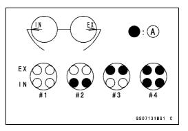
★If the valve clearance is not within the specified range, first record the clearance, and then adjust it.
