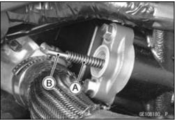
• Remove the mounting bolts [A] and take off the camshaft chain tensioner body [B].
