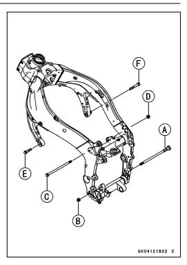
OSecond, tighten the left front engine mounting bolt [A].
