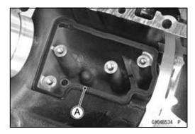
Apply a non-permanent locking agent to the threads of the bolts [A] and tighten them.
