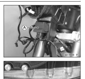
Oxygen Sensor [A] (Equipped Models)
