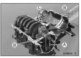
• Apply liquid gasket [A] to the mating surface of the lower crankcase half.
