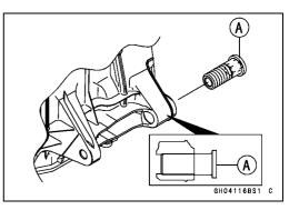
• Install the adjusting collar [A] to the frame until end of the threads.
