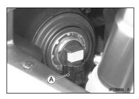
• Turn the headlight bulb [A] counterclockwise and pull out the bulb from the headlight.
