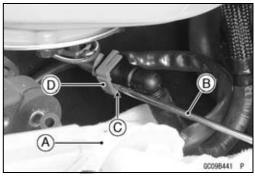
Turn [A] the driver to disconnect the joint lock [B].
