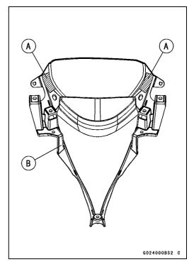
OInsert the slots [A] onto the hook portions. OTighten the screws [B].
