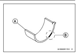
• Install the new inserts in the connecting rod and check insert/crankpin clearance with the plastigage.
