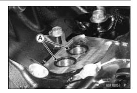
• Install the oil cooler/oil filter case.
