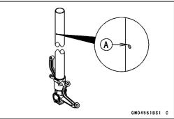
Drain the fork oil into a suitable container [A].
