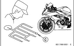
Even when the DFI system is operating normally, the warning indicator light (LED) and FI warning symbol may blink under strong electrical interference. Additional measures are not required. Turn the ignition switch OFF to stop the indicator light and symbol.
