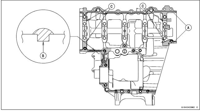
• Fit the lower crankcase half to the upper crankcase half.
