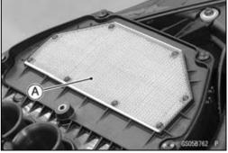
Install a new element [A] so that the screen side [B] faces upward.
