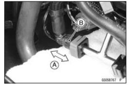
For Secondary Fuel Hose (Throttle Body Assy ~ Nozzle Assy)
