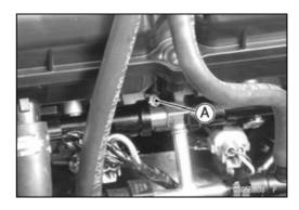
★If any one vacuum measurement is out of the standard measurement after left and right synchronization, turn in the bypass screws [A] until it seats fully but not tightly. Rear View [B]
