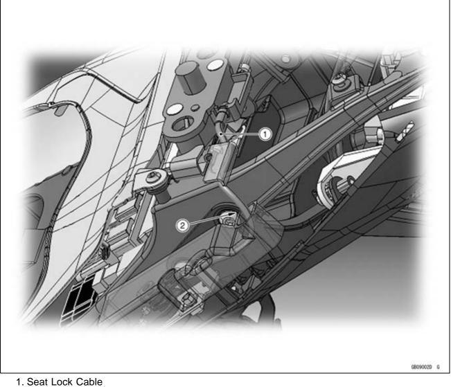
2. Run the seat lock cable into the hole of the seat lock cover.
