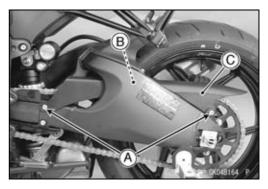
Remove: Bolts [A] Quick Rivet [B] Chain Cover [C]
