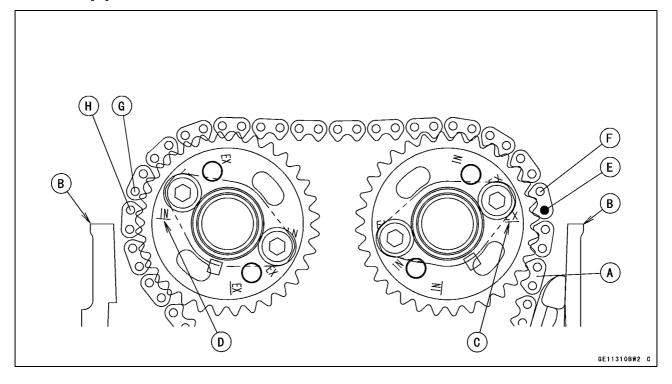
• Apply molybdenum disulfide oil solution [A] to all cam lobes, journals and thrust journals.
