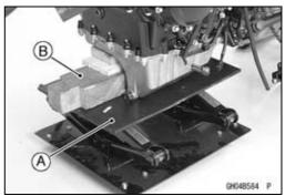
• Disconnect the sidestand switch lead connector [A].
