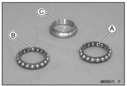
Remove the lower bearing inner race (with its grease seal)
