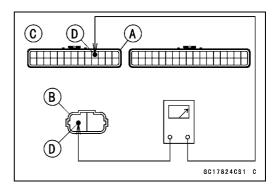
Wiring Continuity Inspection (Secondary Fuel Injectors) ECU Connector [A] ←→ Secondary Fuel Injector Connector [E]
