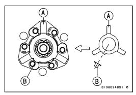
OSecond Torque Limiter Spring [A] Tang [B]
