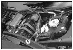
• Connect the test light [A] (12 V 3.4 W bulb in a socket with leads) and the 12 V battery [B] to the fuel pump lead connector [C].
