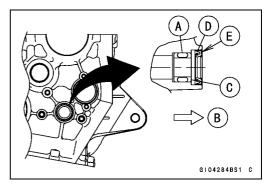
• Install the oil passage nozzle [A] in the lower crankcase, and tighten it.
