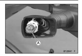
• Insert the new bulb [A] by aligning its left and right pins [B] with the left and right grooves [C] in the socket, and turn C
