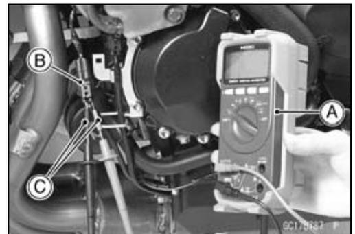
**Oxygen Sensor #2 Output Voltage**
