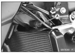
Move the radiator right ward [A] to clear the frame projection [B].
