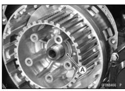
• Install the washer so that the "OUTSIDE" mark [A] faces outward.
