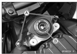
• Using a small chisel [A] or punch, turn out the Torx bolts.
