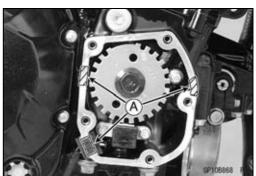
• Replace the O-ring [A] in the crankshaft sensor cover with a new one.
