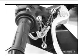
Remove: Bolts [A] Throttle Pulley Cover [B]
