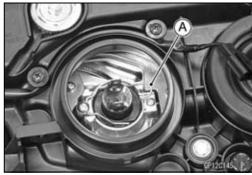
• Install the dust covers [A] so that align the arrow marks [B] and slits [C] on the headlight body.
