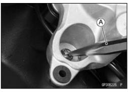
Remove: Bolts [A] Ignition Switch [B]
