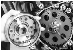
• Install the alternator rotor [A] while turning [B] the starter clutch gear [C] clockwise.
