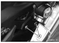
Remove: Quick Rivets [A] Mud Guard [B]
